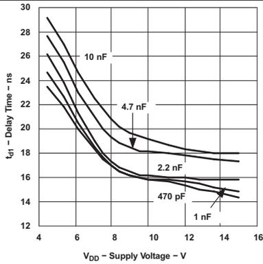
Figure 15. Delay Time ( $t_{D1}$ ) vs Supply Voltage (UCC27423)
