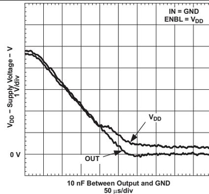
Figure 20. Output Behavior vs Supply Voltage (Inverting)
