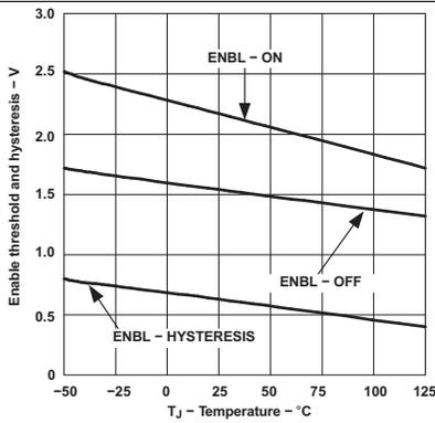
Figure 17. Enable Threshold and Hysteresis vs Temperature
