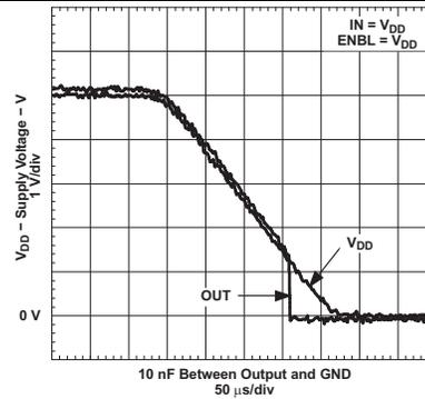
Figure 24. Output Behavior vs VDD (Noninverting)
