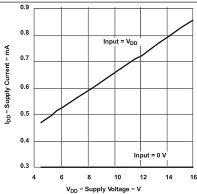
Figure 9. Supply Current vs Supply Voltage (UCC274323)
