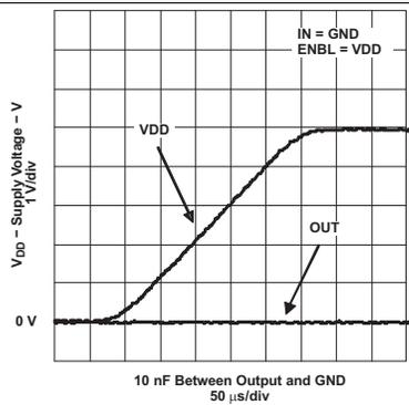
Figure 25. Output Behavior vs VDD (Noninverting)
