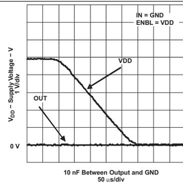
Figure 26. Output Behavior vs VDD (Noninverting)
