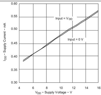
Figure 10. Supply Current vs Supply Voltage (UCC27424)
