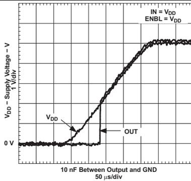
Figure 23. Output Behavior vs VDD (Noninverting)
