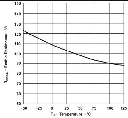
Figure 18. Enable Resistance vs Temperature
