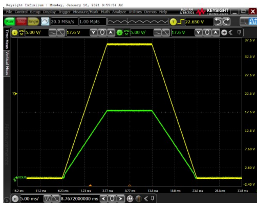
G = 1, V_{IN} = 4 V during Power On and Off Yellow: + V_S ; Green: Output
