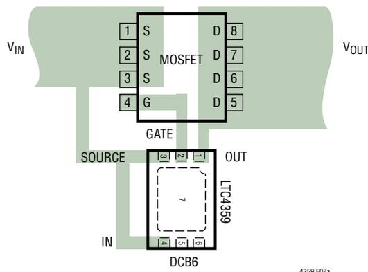
Figure 7a. Layout, DCB6 Package
