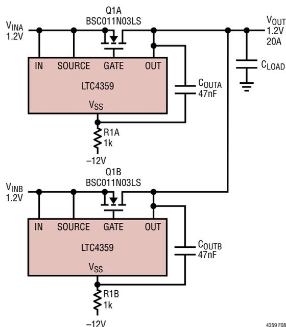
Figure 8. 1.2V Diode-OR
