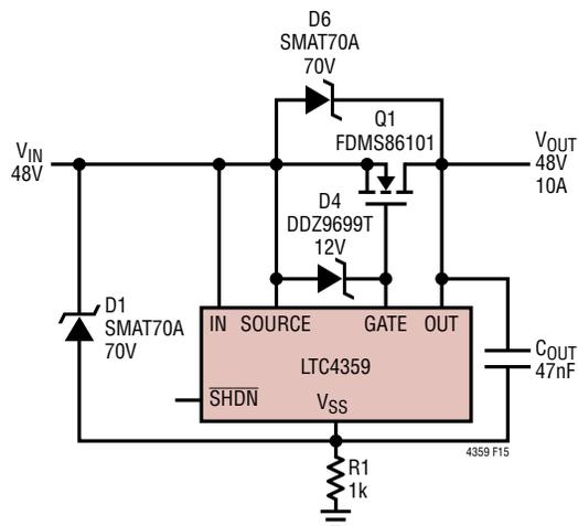
Figure 15. 48V Ideal Diode without Reverse Input Protection
