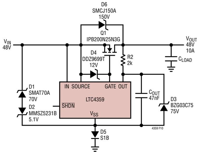
**Figure 10. 48V Ideal Diode with Reverse Input Protection**
