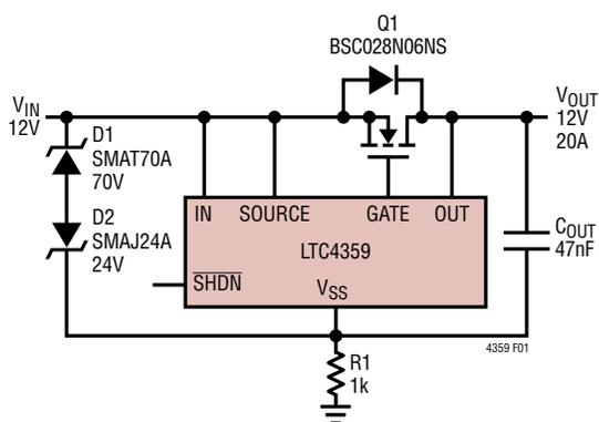
Figure 1. 12V/20A Ideal Diode with Reverse Input Protection
