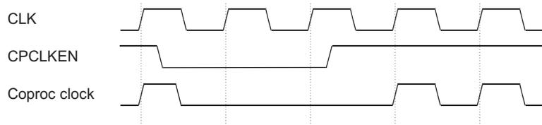
**Figure 8-2 Coprocessor clocking**
