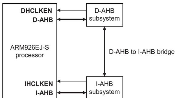
**Figure 6-2 Multi-AHB system example**
