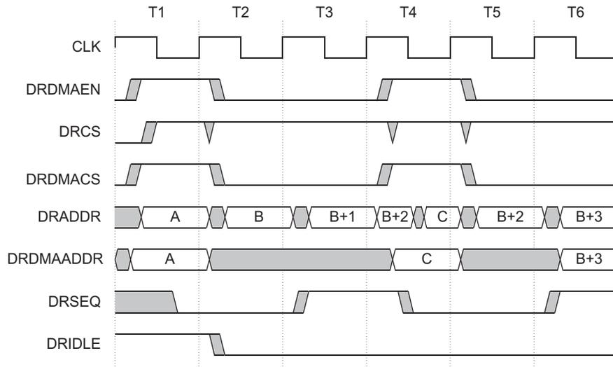
**Figure 5-5 DMA access interaction with normal DTCM accesses**
