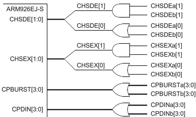
**Figure 8-10 Arrangement for connecting two coprocessors**
