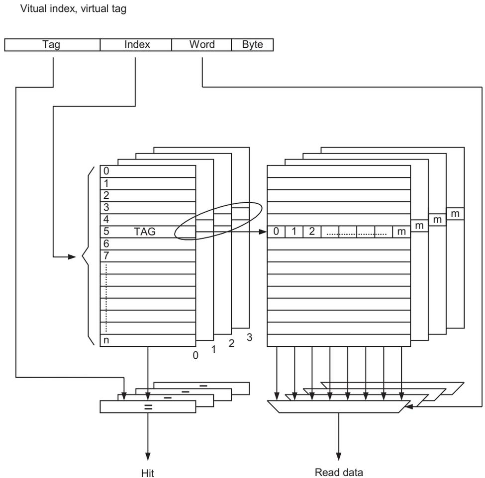
**Figure 4-1 Generic virtually indexed virtually addressed cache**
