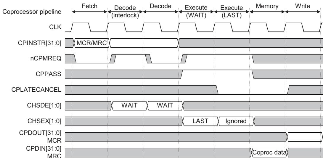
Figure 8-5 Interlocked MCR
