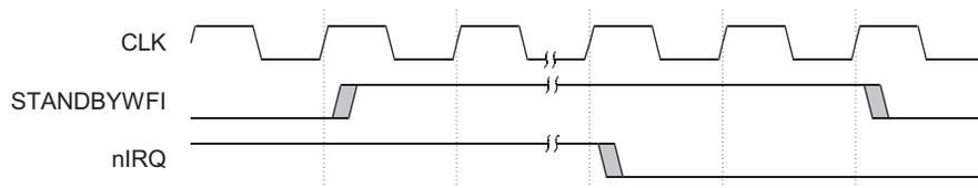
Figure 12-1 Deassertion of STANDBYWFI after an IRQ interrupt
