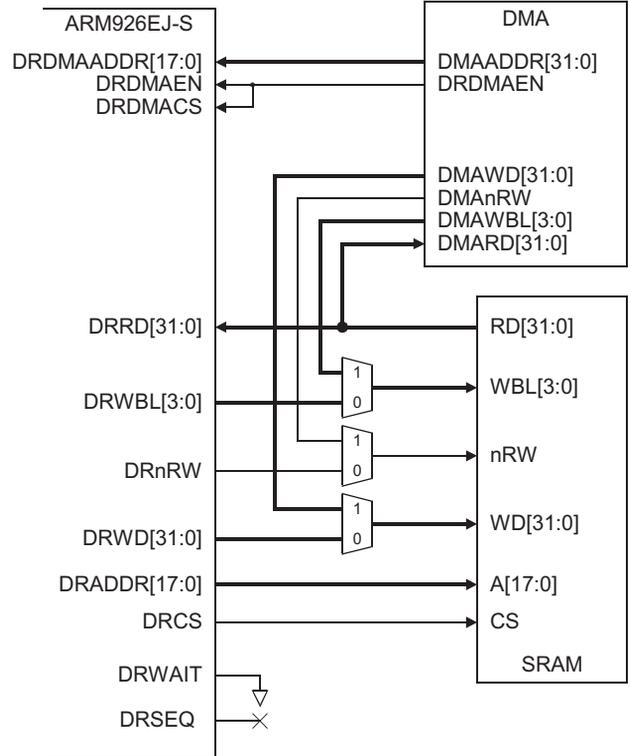
Figure 5-18 TCM subsystem that uses the DMA interface
