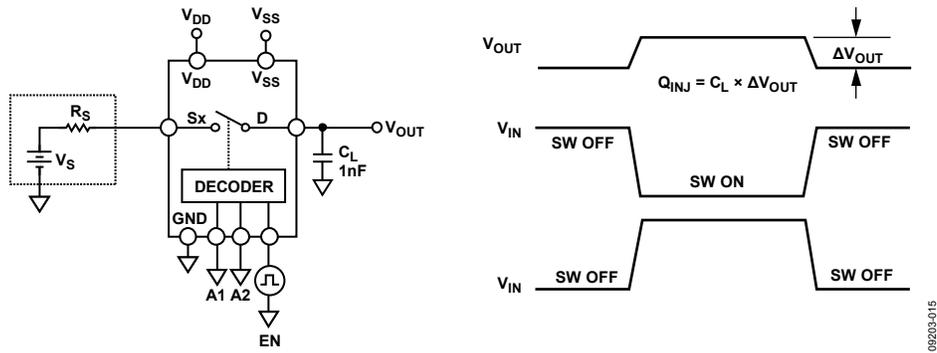
Figure 33. Charge Injection
