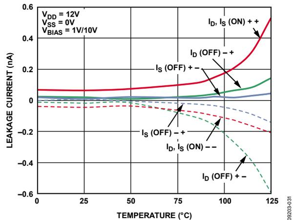
Figure 14. Leakage Currents vs. Temperature, 12 V Single Supply
