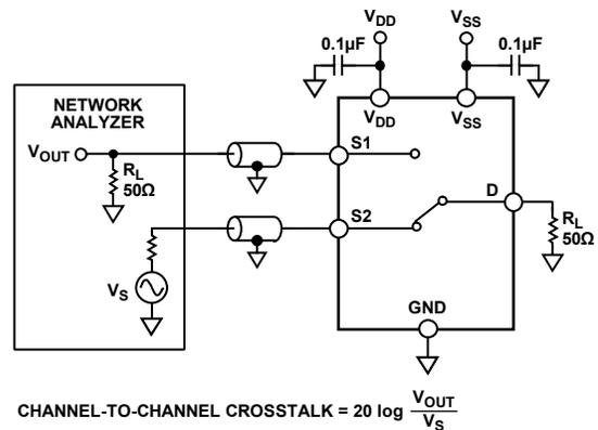
$$\text{CHANNEL-TO-CHANNEL CROSSTALK} = 20 \log \frac{V_{\text{OUT}}}{V_s}$$
