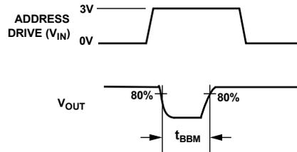
Figure 31. Break-Before-Make Time Delay
