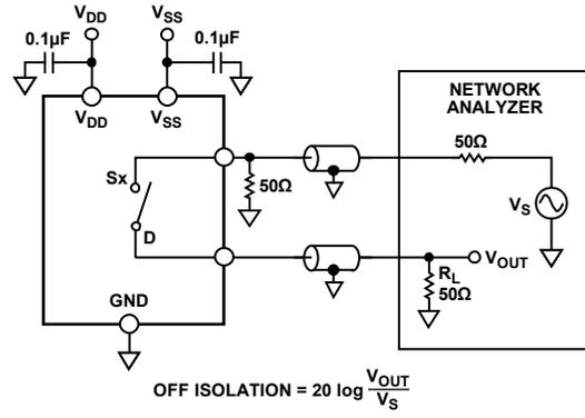
$$\text{OFF ISOLATION} = 20 \log \frac{V_{\text{OUT}}}{V_s}$$
