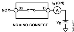
Figure 25. On Leakage
