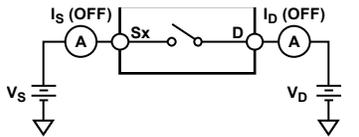
Figure 24. Off Leakage
