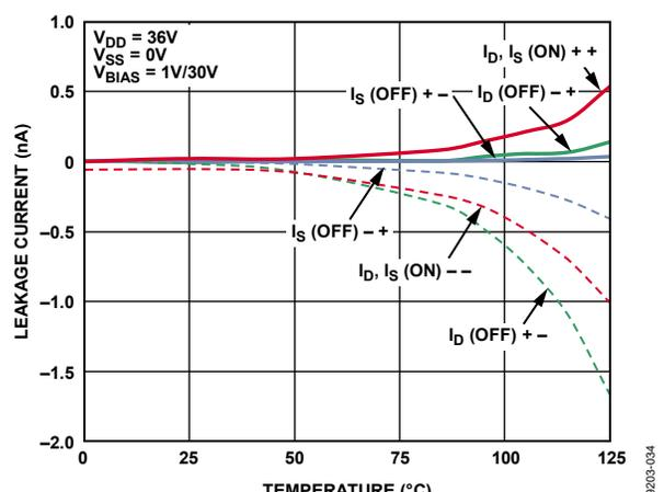
Figure 15. Leakage Currents vs. Temperature, 36 V Single Supply
