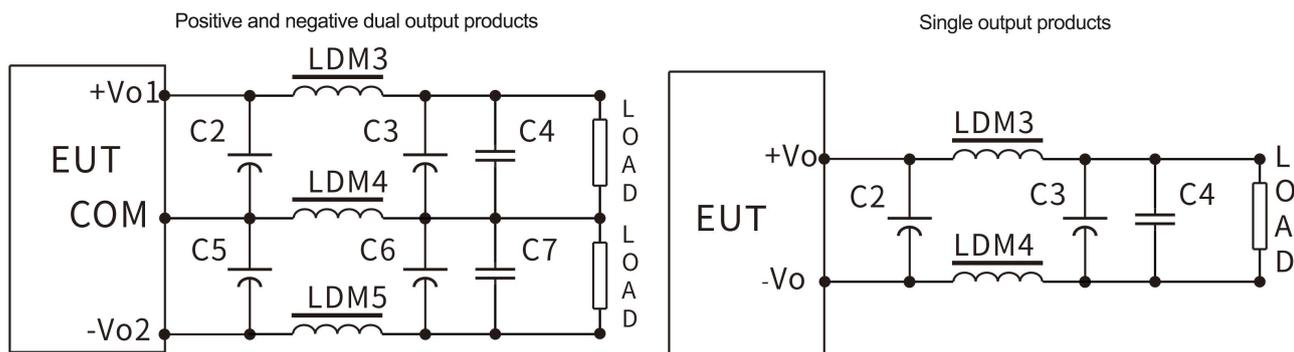
When the requirements for ripple & noise are general, it is recommended to use only C2 and C5 for the periphery;
