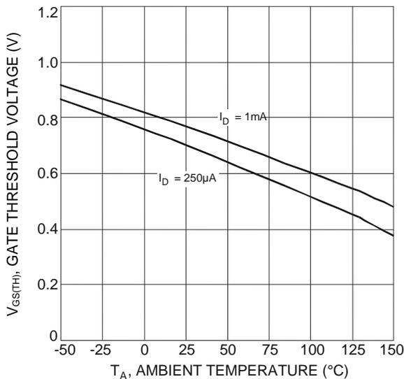
Fig. 9 Gate Threshold Variation vs. Ambient Temperature
