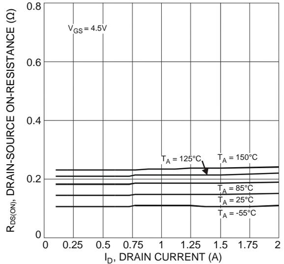
Fig. 6 Typical On-Resistance vs. Drain Current and Temperature
