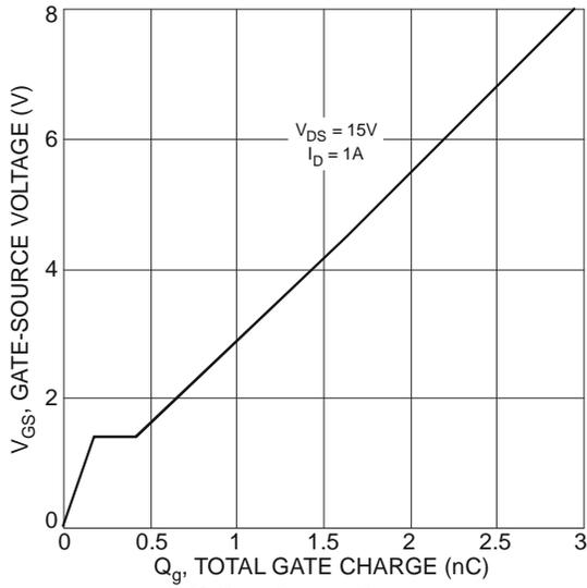
Fig. 13 Gate-Charge Characteristics
