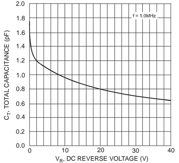
Figure 4 Total Capacitance vs. Reverse Voltage, Per Element
