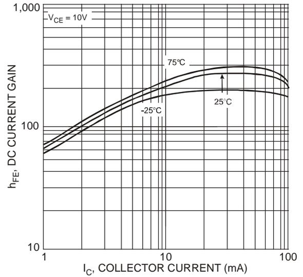
Fig. 2 Typical DC Current Gain vs. Collector Current
