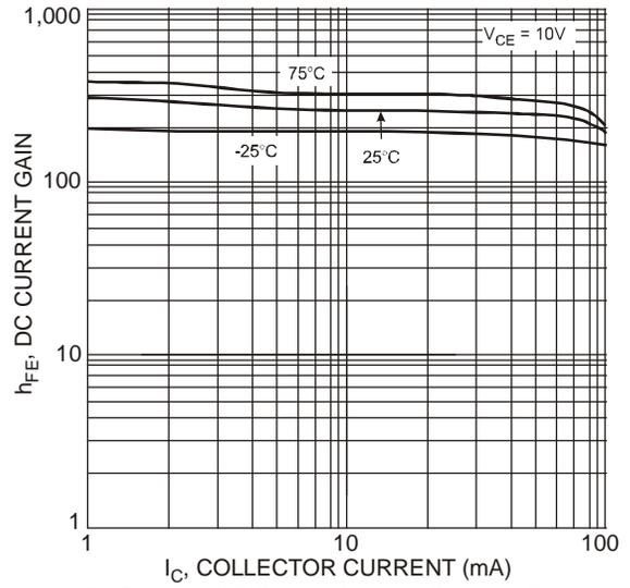
Fig.8 Typical DC Current Gain vs. Collector Current
