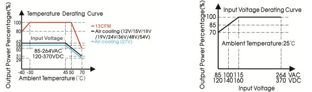
Note: With an AC input voltage between 85-115VAC and a DC input between 120-160VDC the output power must be derated as per the temperature derating curves.
