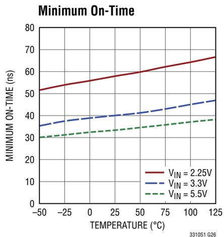
**TYPICAL PERFORMANCE CHARACTERISTICS**  $T_A = 25^\circ\text{C}$ ,  $V_{IN} = 3.3\text{V}$ , unless otherwise noted.
