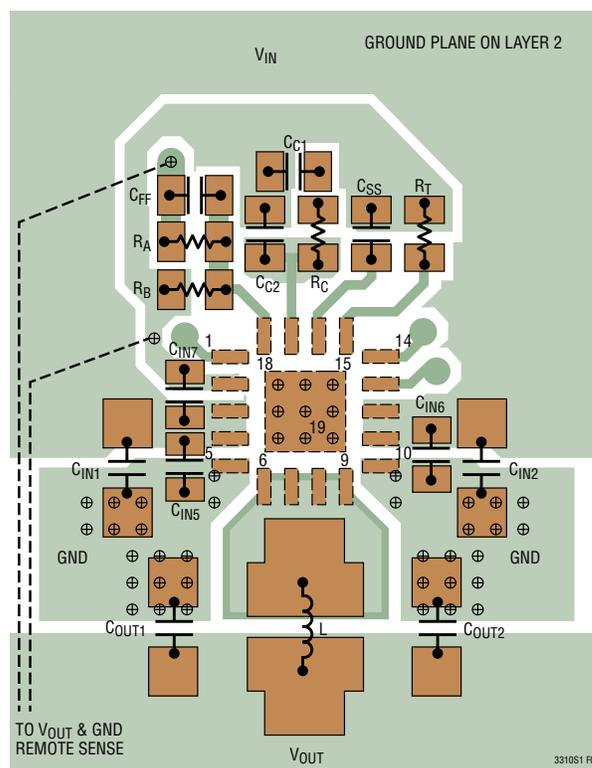
Figure 5. Recommended PCB Layout for the LTC3310
