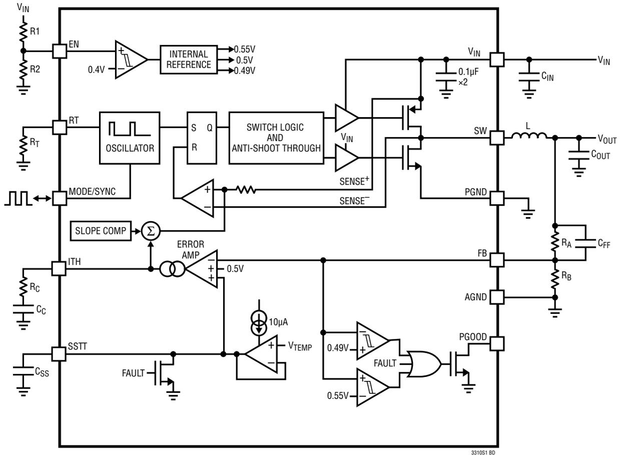
Note 1: On the LTC3310S-1 the  $R_A$  and  $R_B$  resistors are internal.
