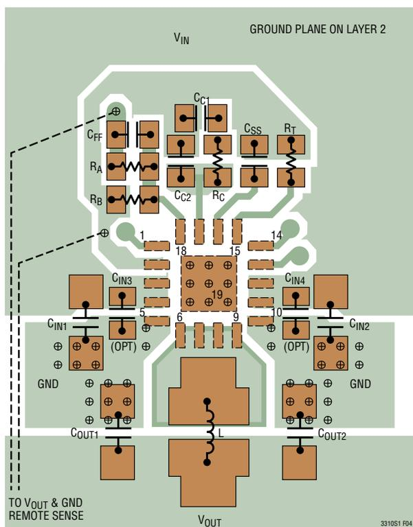
Figure 4. Recommended PCB Layout for the LTC3310S
