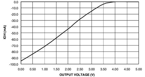
**OUTPUT SOURCE CURRENT VS. SUPPLY VOLTAGE**
