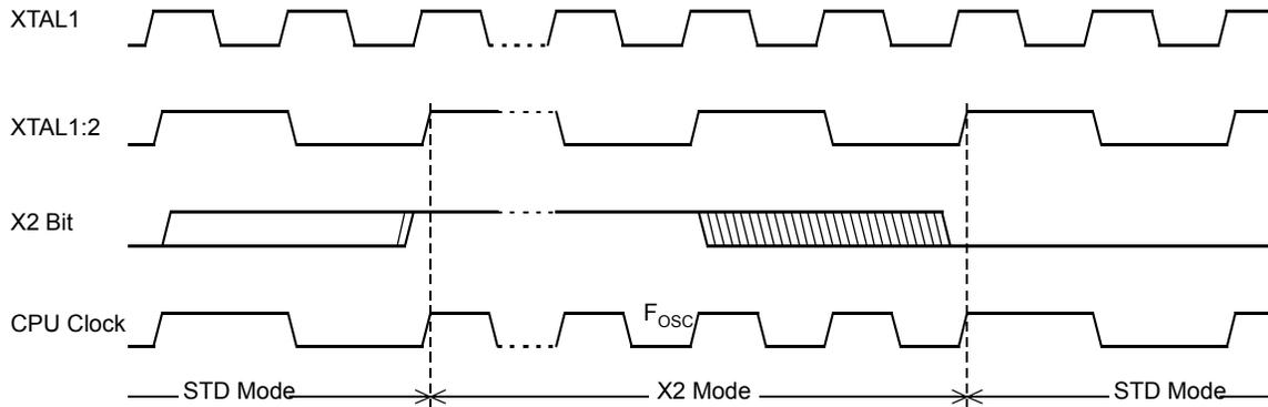
The X2 bit in the CKCON0 register (see Table 16) allows a switch from 12 clock periods per instruction to 6 clock periods and vice versa. At reset, the speed is set according to X2 bit of Hardware Security Byte (HSB). By default, Standard mode is active. Setting the X2 bit activates the X2 feature (X2 mode).
