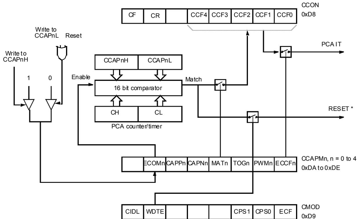
Before enabling ECOM bit, CCAPnL and CCAPnH should be set with a non zero value, otherwise an unwanted match could happen. Writing to CCAPnH will set the ECOM bit.
