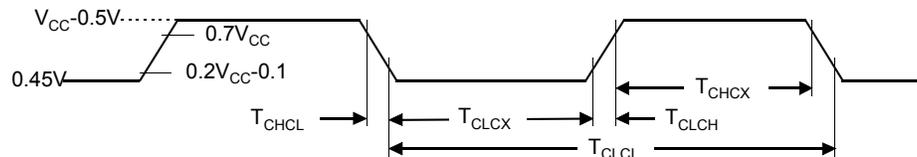
**AC Testing Input/Output Waveforms**
