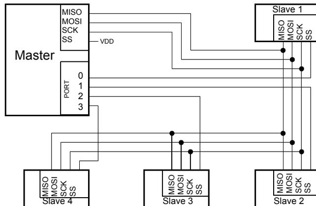
The Master device selects the individual Slave devices by using four pins of a parallel port to control the four  $\overline{SS}$  pins of the Slave devices.
