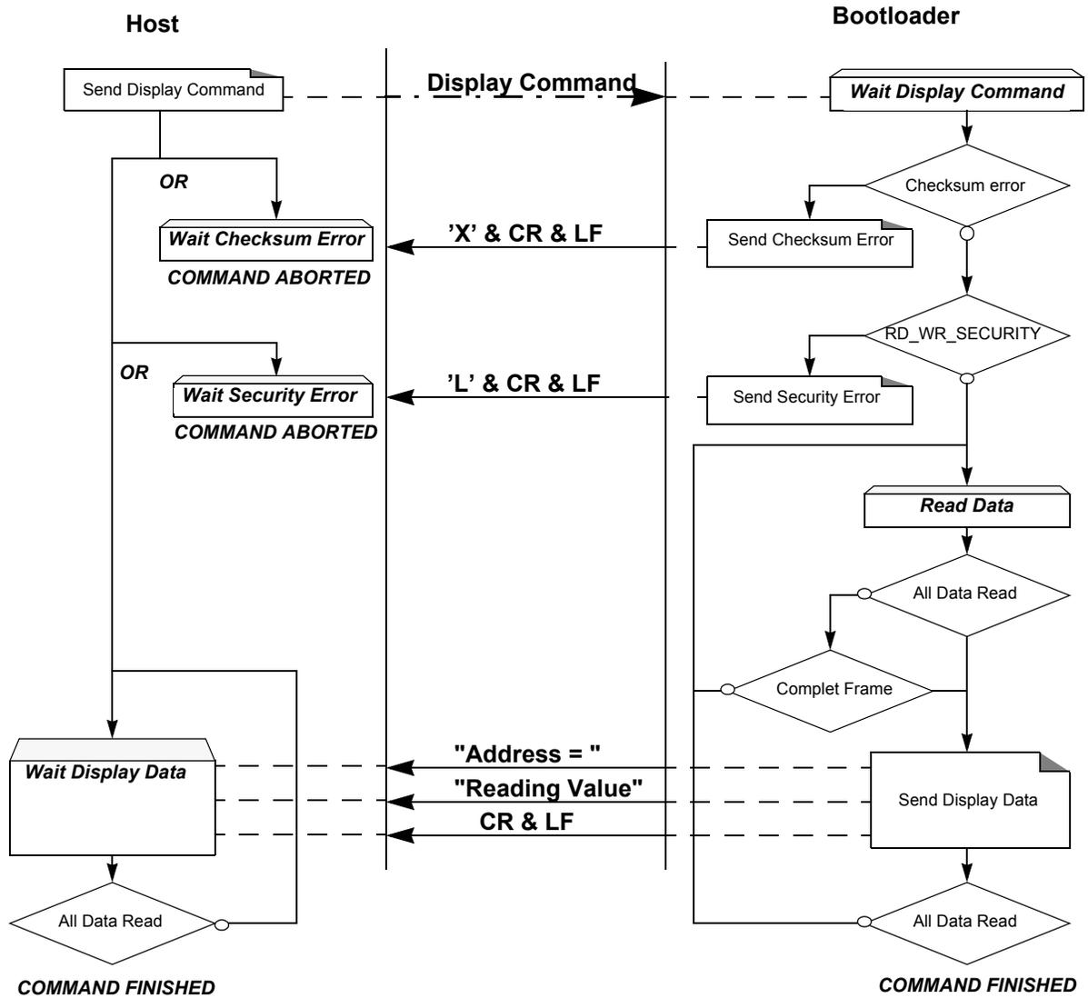
Note: The maximum size of block is 400h. To read more than 400h bytes, the Host must send a new command.
