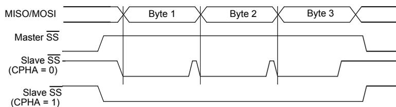
As shown in Figure 32, the first SCK edge is the MSB capture strobe. Therefore, the Slave must begin driving its data before the first SCK edge, and a falling edge on the  $\overline{SS}$  pin is used to start the transmission. The  $\overline{SS}$  pin must be toggled high and then low between each Byte transmitted (Figure 34).
