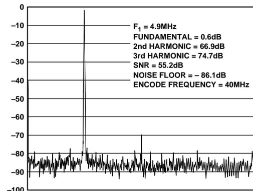
Figure 39. FFT Output of Circuit in Figure 38
