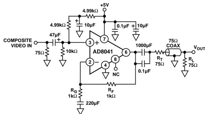
Figure 42. Single Supply Composite Video Line Driver
