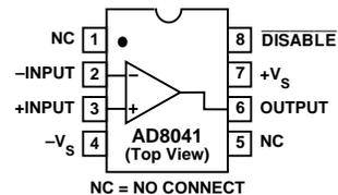
The output voltage swing extends to within 50 mV of each rail, providing the maximum output dynamic range. Additionally, it features gain flatness of 0.1 dB to 30 MHz while offering differential gain and phase error of 0.03% and 0.03° on a single +5 V supply. This makes the AD8041 ideal for professional video electronics such as cameras, video switchers or any high speed portable equipment. The AD8041's low distortion and fast settling make it ideal for buffering high speed A-to-D converters.
