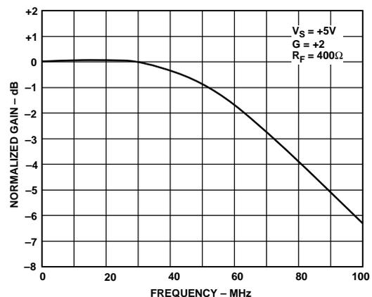
Figure 2. Frequency Response: Gain =  $+2$ ,  $V_S = +5$  V
