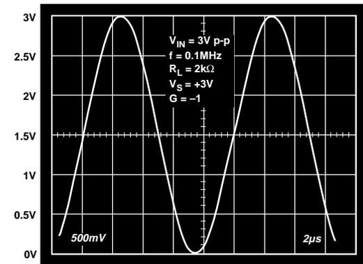
Figure 31. Output Swing,  $V_S = +3\text{ V}$ ,  $V_{IN} = 3\text{ V p-p}$
