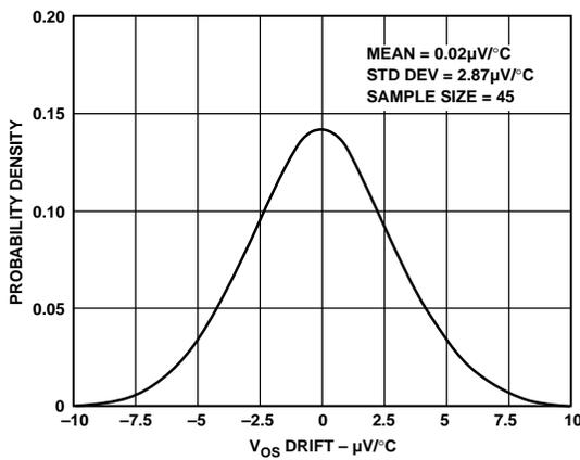
Figure 5.  $V_{OS}$  Drift Over -40°C to +85°C
