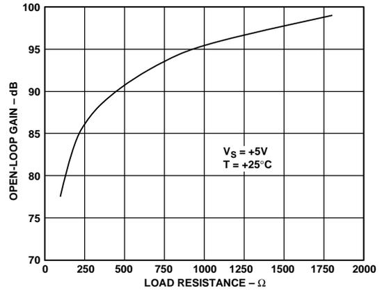
Figure 7. Open-Loop Gain vs.  $R_L$  to +25°C
