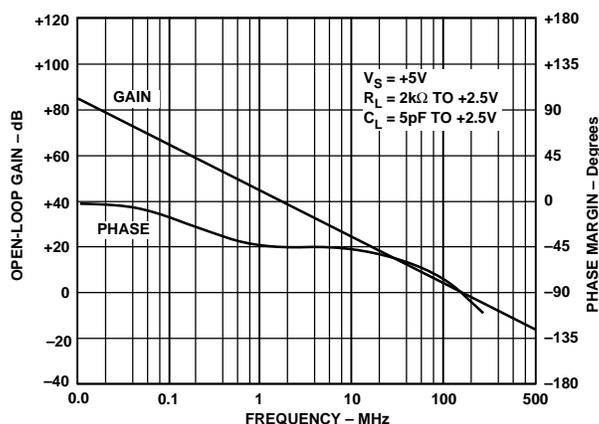
Figure 15. Open-Loop Gain and Phase Margin vs. Frequency
