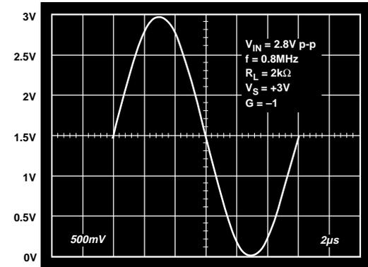
Figure 32. Output Swing,  $V_S = +3\text{ V}$ ,  $V_{IN} = 2.8\text{ V p-p}$
