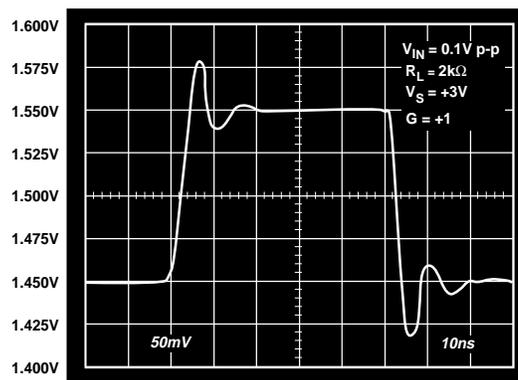
Figure 27. Pulse Response,  $V_S = +3 V$
