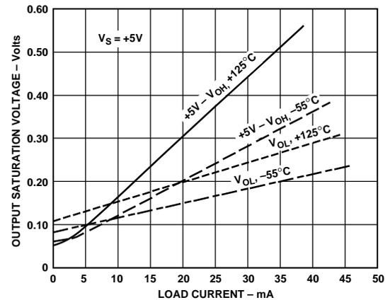
Figure 21. Output Saturation Voltage vs. Load Current
