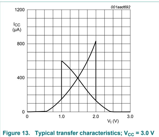
Figure 13. Typical transfer characteristics;  $V_{CC} = 3.0 V$
