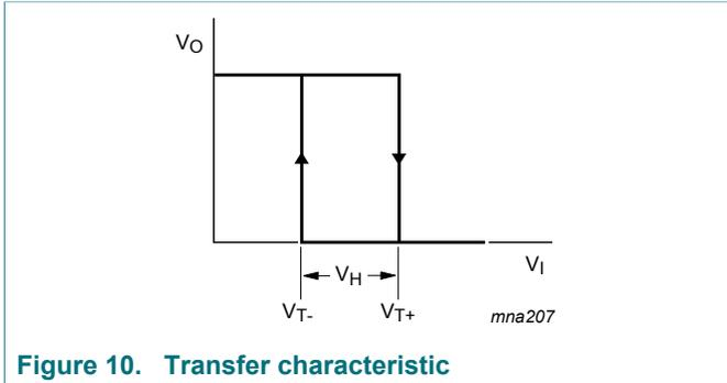
Figure 10. Transfer characteristic
