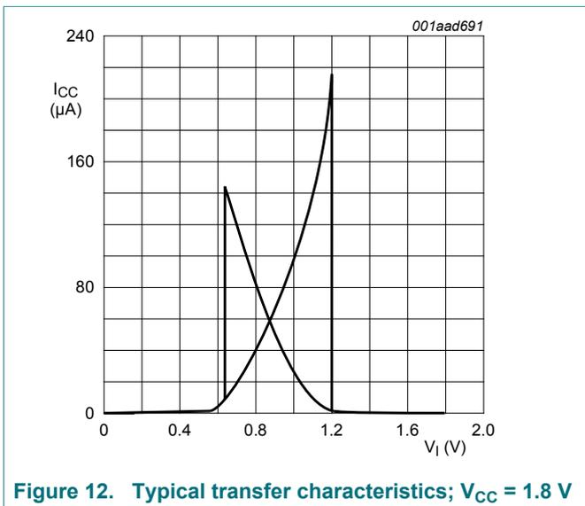
Figure 12. Typical transfer characteristics;  $V_{CC} = 1.8 V$
