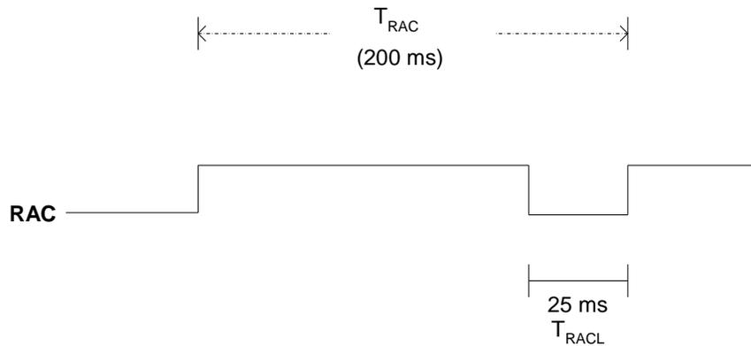
FIGURE 2: RAC TIMING WAVEFORM DURING NORMAL OPERATION
