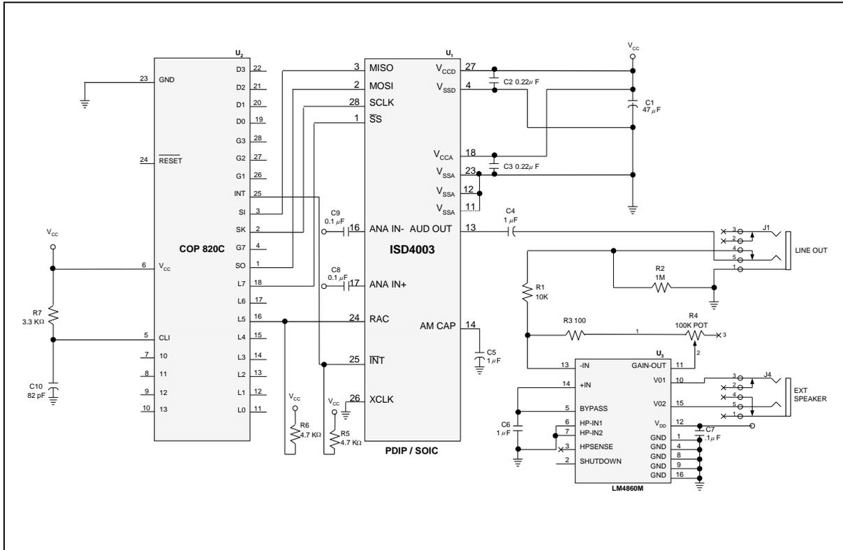
FIGURE 11: APPLICATION EXAMPLE USING SPI PORT ON MICROCONTROLLER
