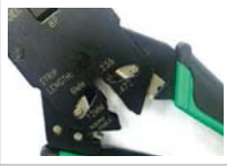
Stripping twisted pair round cable
