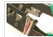
Strips flat telephone wire
