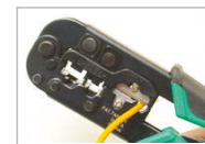
Strips twisted pair wire
