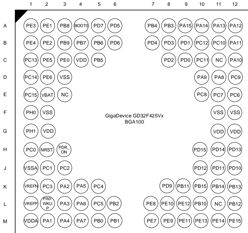
Figure 2-2. GD32F425Vx BGA100 pinouts
