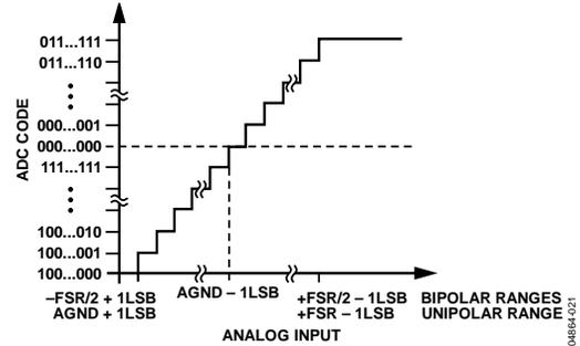
Figure 27. Twos Complement Transfer Characteristic (Bipolar Ranges)
