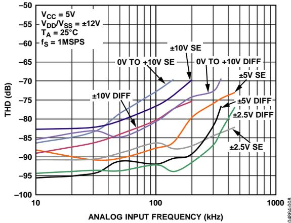
Figure 10. THD vs. Analog Input Frequency for Single-Ended (SE) and True Differential Mode (Diff) at 5 V<sub>CC</sub>
