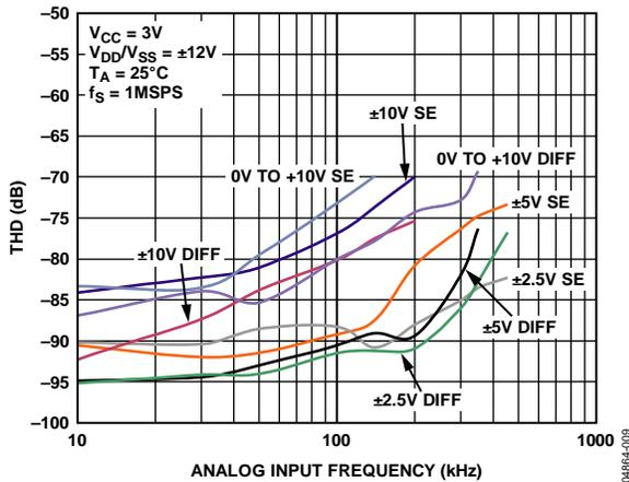
Figure 11. THD vs. Analog Input Frequency for Single-Ended (SE) and True Differential Mode (Diff) at 3 V<sub>CC</sub>
