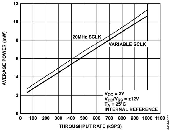
Figure 49. Power vs. Throughput Rate with 3 V  $V_{CC}$
