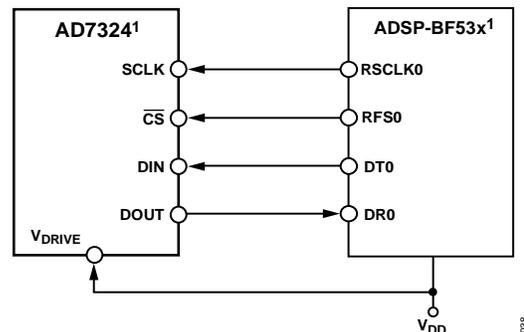
Figure 53. Interfacing the AD7324 to the ADSP-BF53x
