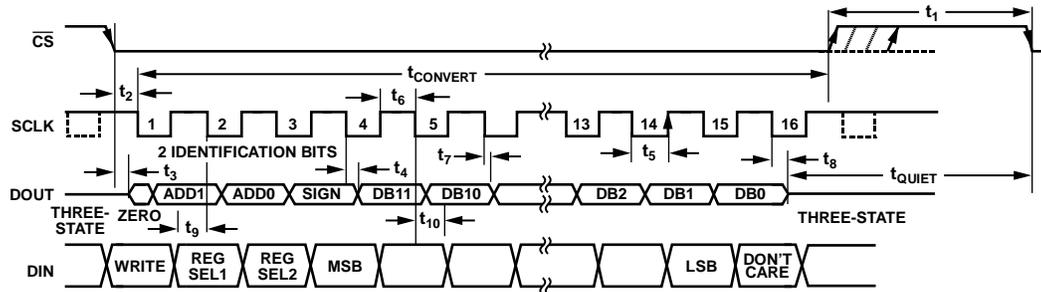
Figure 51. Serial Interface Timing Diagram (Control Register Write)
