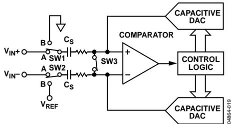
Figure 25. ADC Differential Configuration During Acquisition Phase
