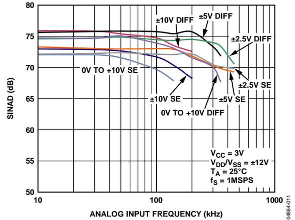
Figure 13. SINAD vs. Analog Input Frequency for Single-Ended (SE) and Differential Mode (Diff) at 3 V<sub>CC</sub>
