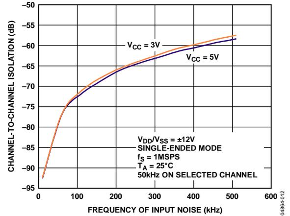
Figure 14. Channel-to-Channel Isolation
