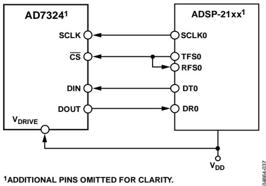
Figure 52. Interfacing the AD7324 to the ADSP-21xx
