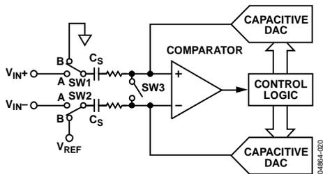
Figure 26. ADC Differential Configuration During Conversion Phase
