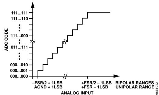
Figure 28. Straight Binary Transfer Characteristic (Bipolar Ranges)
