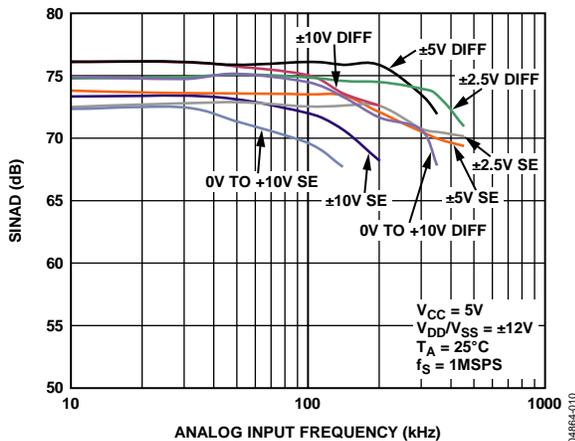
Figure 12. SINAD vs. Analog Input Frequency for Single-Ended (SE) and Differential Mode (Diff) at 5 V<sub>CC</sub>
