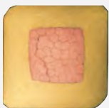
Micrograph of a square crimp
