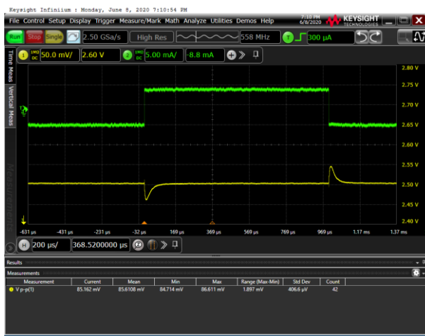
Figure 11. Load Transient, \pm 5\text{ mA} , V_{IN} = 5\text{ V} , C_{IN} = 1\ \mu\text{F} , C_{OUT} = 1\ \mu\text{F} , 50\text{ mV/div}
