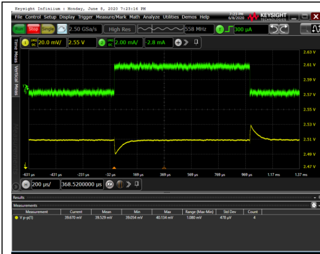
Figure 13. Load Transient, \pm 2\text{ mA} , V_{IN} = 5\text{ V} , C_{IN} = 1\ \mu\text{F} , C_{OUT} = 1\ \mu\text{F} , 20 mV/div
