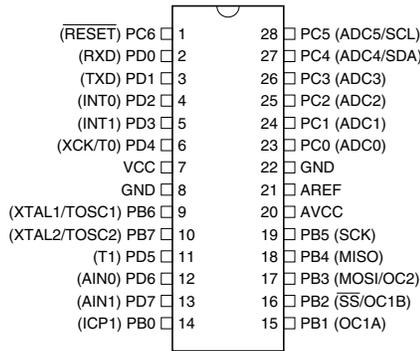
**TQFP Top View**
