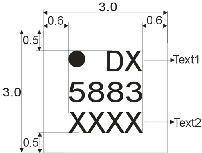
Figure 4. Chip Marking
