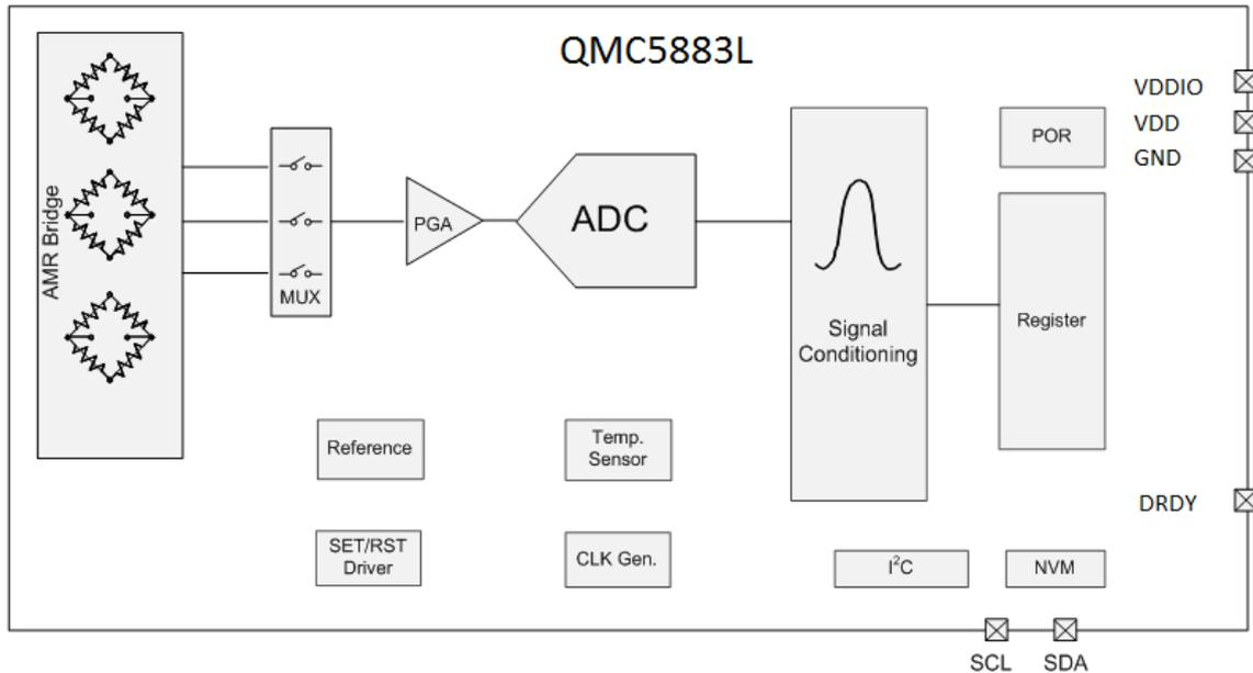
Figure 1. Block Diagram
