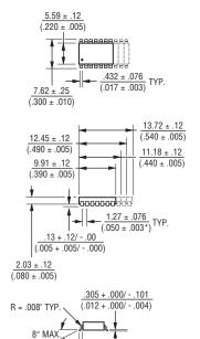
Lead coplanarity .102mm (.004 inch) max. at mounting surface.
