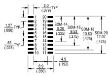
NOTE: Land pattern dimensions are based on design rules established by the Institute for Inter-connecting and Packaging Electronic Circuits in IPC-SM-782.
