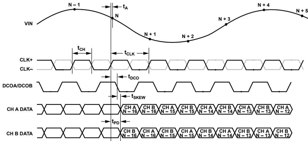
Figure 3. CMOS Interleaved Output Mode Data Output Timing
