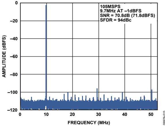
Figure 23. Single-Tone FFT with  $f_{IN} = 9.7$  MHz
