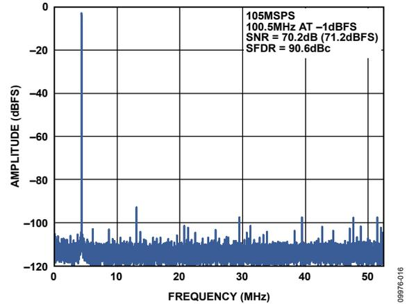
Figure 26. Single-Tone FFT with  $f_{IN} = 100.5$  MHz
