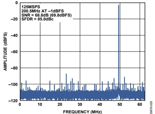
Figure 13. Single-Tone FFT with  $f_{IN} = 200.5$  MHz
