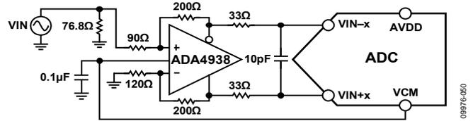
Figure 44. Differential Input Configuration Using the ADA4938-2
