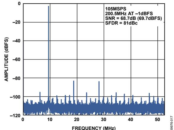
Figure 27. Single-Tone FFT with  $f_{IN} = 200.5$  MHz
