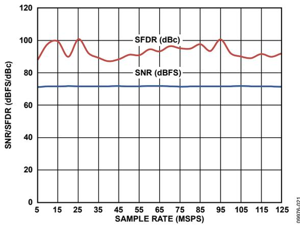
Figure 19. SNR/SFDR vs. Sample Rate with AIN = 70 MHz
