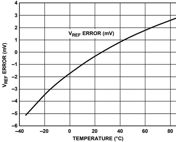
Figure 50. Typical V<sub>REF</sub> Drift
