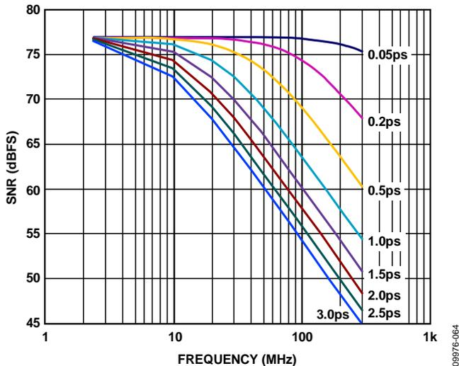
Figure 58. SNR vs. Input Frequency and Jitter
