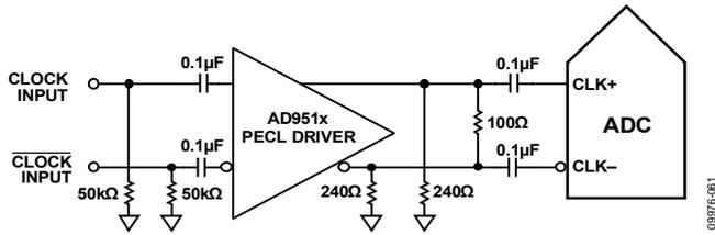
Figure 54. Differential PECL Sample Clock (Up to 1 GHz)
