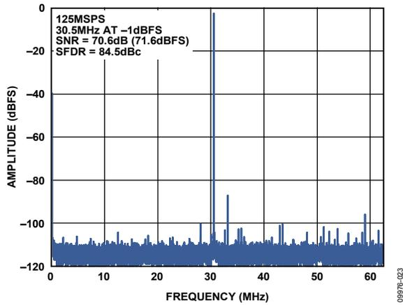
Figure 10. Single-Tone FFT with  $f_{IN} = 30.5$  MHz
