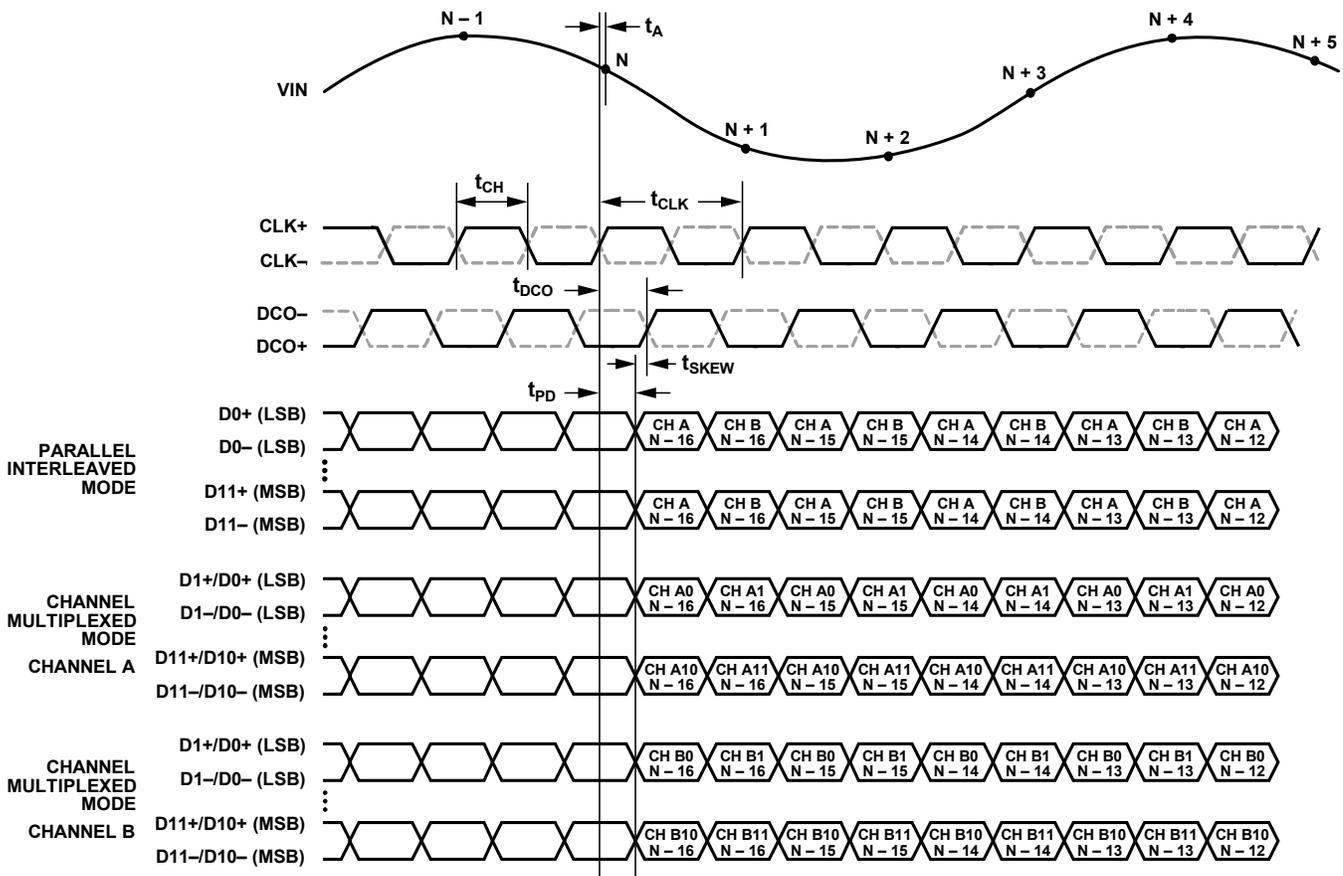
Figure 4. LVDS Modes for Data Output Timing
