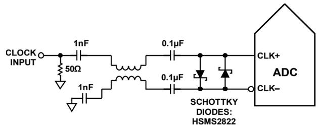
Figure 53. Balun-Coupled Differential Clock (Up to 1 GHz)
