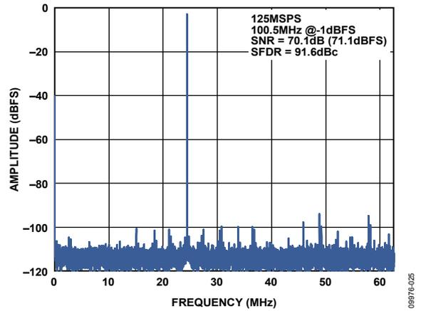
Figure 12. Single-Tone FFT with  $f_{IN} = 100.5$  MHz
