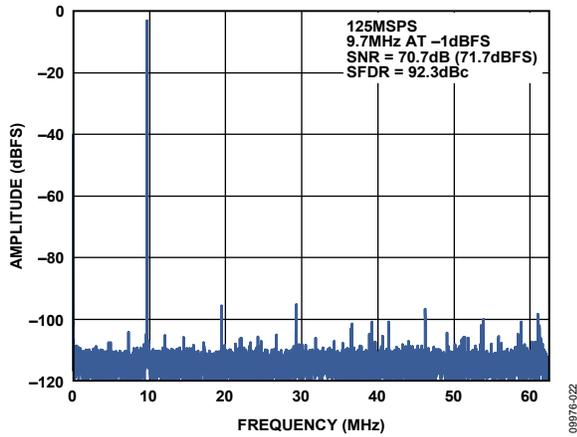
Figure 9. Single-Tone FFT with  $f_{IN} = 9.7$  MHz
