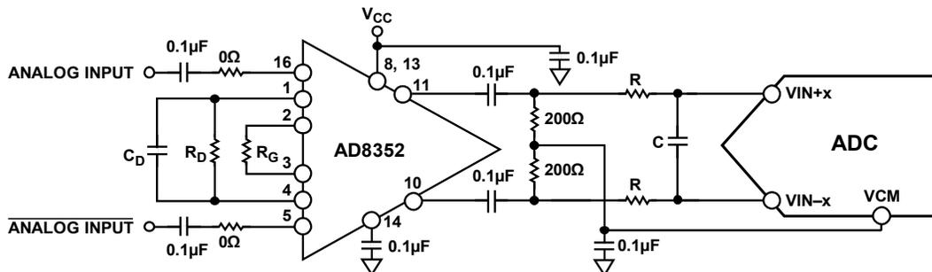
Figure 47. Differential Input Configuration Using the AD8352
