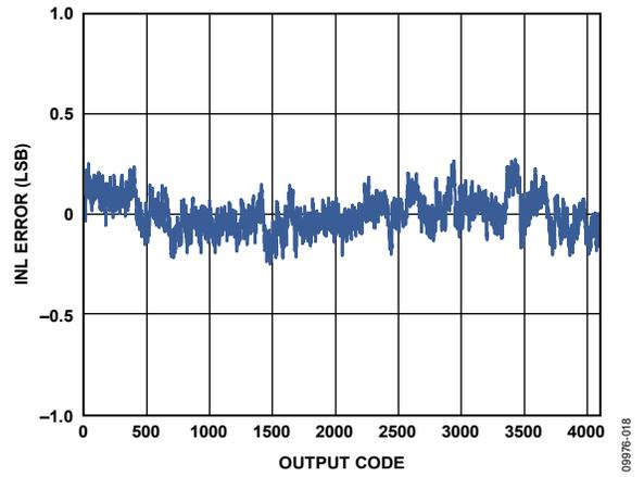
Figure 22. INL Error with  $f_{IN} = 9.7$  MHz
