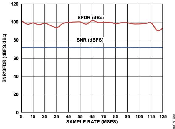
Figure 16. SNR/SFDR vs. Sample Rate with AIN = 9.7 MHz
