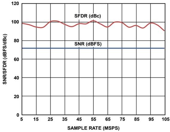
Figure 29. SNR/SFDR vs. Sample Rate with AIN = 9.7 MHz
