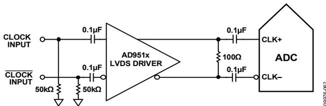
Figure 55. Differential LVDS Sample Clock (Up to 1 GHz)
