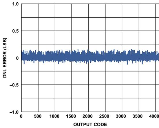
Figure 30. DNL Error with  $f_{IN} = 9.7$  MHz
