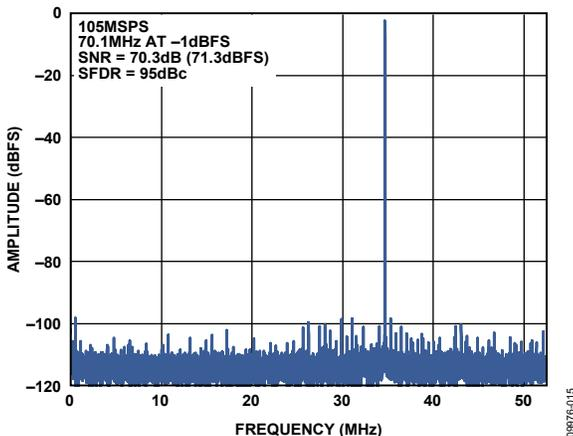
Figure 25. Single-Tone FFT with  $f_{IN} = 70.1$  MHz
