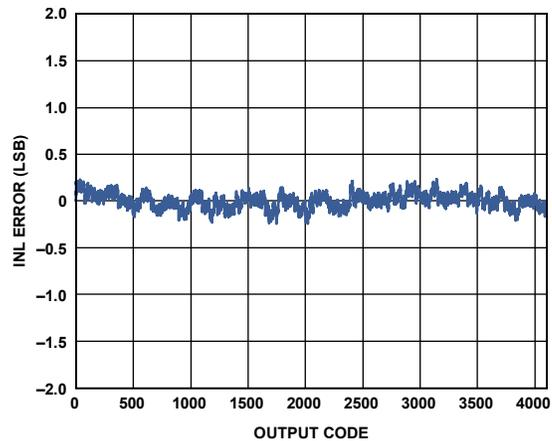
Figure 33. INL Error with  $f_{IN} = 9.7$  MHz
