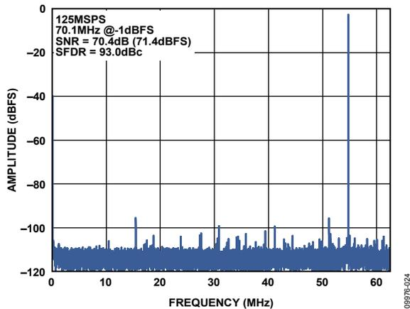
Figure 11. Single-Tone FFT with  $f_{IN} = 70.1$  MHz
