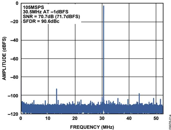
Figure 24. Single-Tone FFT with  $f_{IN} = 30.5$  MHz
