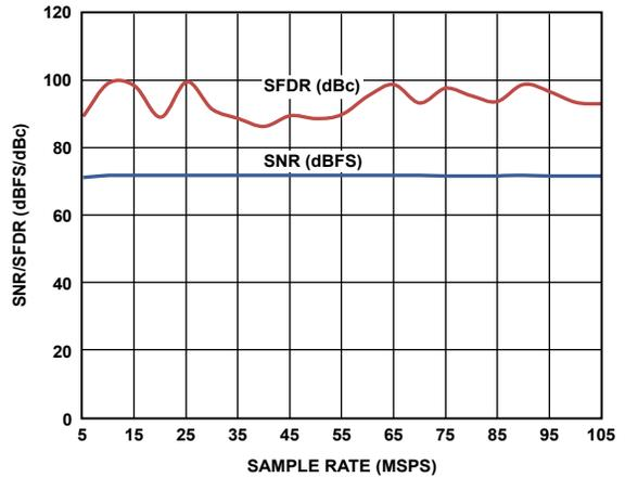
Figure 32. SNR/SFDR vs. Sample Rate with AIN = 70.1 MHz
