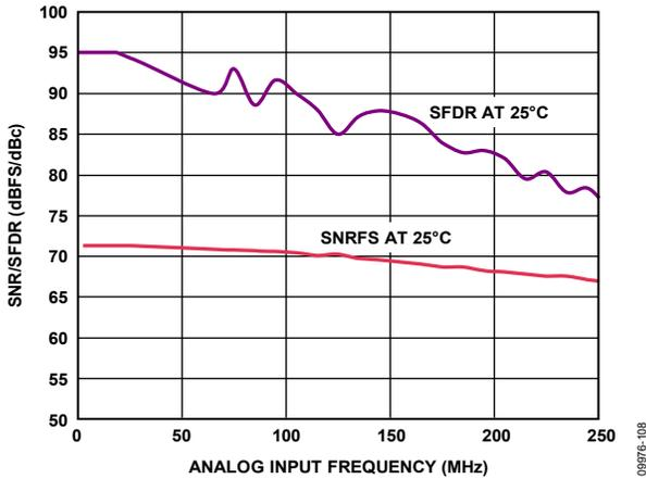
Figure 15. SNR/SFDR vs. Input Frequency (AIN) with 2 V<sub>p-p</sub> Full Scale
