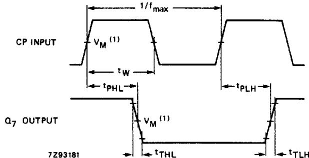
Fig.7 Waveforms showing the clock (CP) to output (Q<sub>7</sub>) propagation delays, the clock pulse width, the output transition times and the maximum clock frequency.
