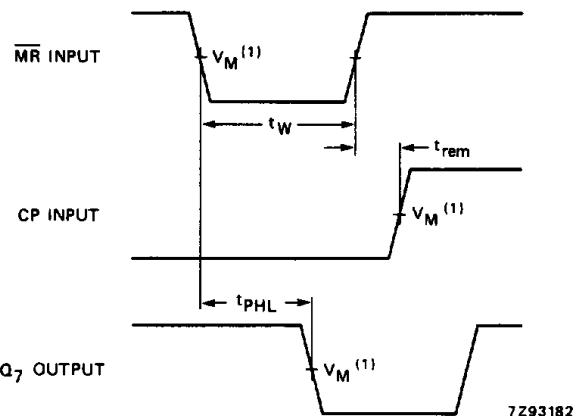
Fig.8 Waveforms showing the master reset (MR) pulse width, the master reset to output (Q<sub>7</sub>) propagation delay and the master reset to clock (CP) removal time.
