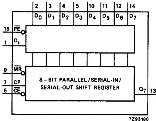
Fig.4 Functional diagram.
