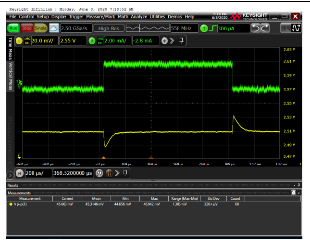
Figure 14. Load Transient, \pm 2\text{ mA} , V_{\text{IN}} = 2.8\text{ V} , C_{\text{IN}} = 1\ \mu\text{F} , C_{\text{OUT}} = 1\ \mu\text{F} , 20 mV/div
