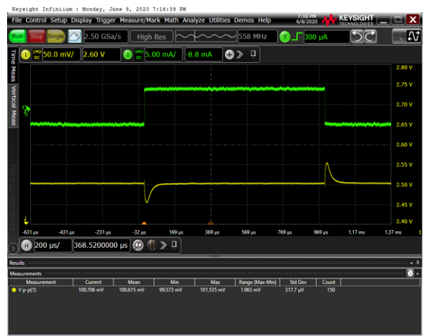
Figure 12. Load Transient, \pm 5\text{ mA} , V_{IN} = 2.8\text{ V} , C_{IN} = 1\ \mu\text{F} , C_{OUT} = 1\ \mu\text{F} , 50\text{ mV/div}
