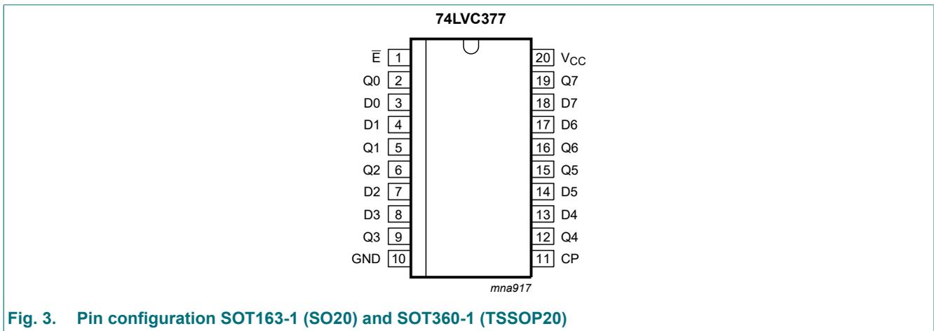
Fig. 3. Pin configuration SOT163-1 (SO20) and SOT360-1 (TSSOP20)
