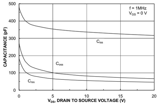
Figure 8. Capacitance Characteristics.
