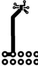
d. 151 °C/W when mounted on a minimum pad of 2 oz copper
