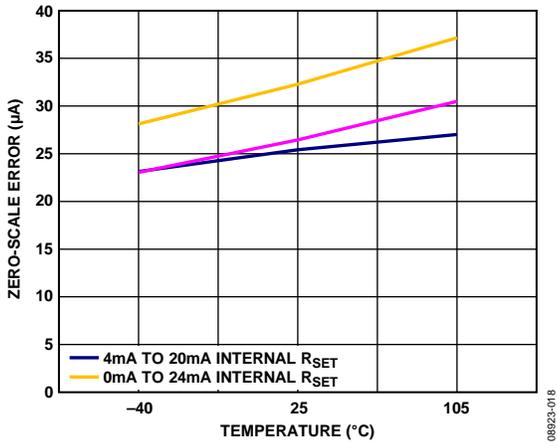
Figure 18. Zero-Scale Error vs. Temperature, Internal R<sub>SET</sub> Sense Resistor
