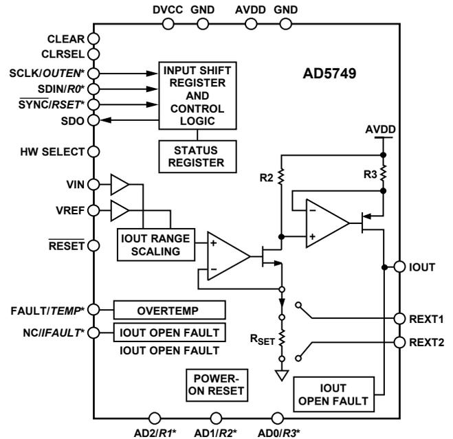
\*DENOTES SHARED PIN. SOFTWARE MODE DENOTED BY REGULAR TEXT, HARDWARE MODE DENOTED BY *ITALIC TEXT*. FOR EXAMPLE, FOR FAULT/TEMP PIN, IN SOFTWARE MODE, THIS PIN TAKES ON FAULT FUNCTION. IN HARDWARE MODE, THIS PIN TAKES ON TEMP FUNCTION.
