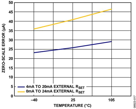
Figure 17. Zero-Scale Error vs. Temperature, External R<sub>SET</sub> Sense Resistor
