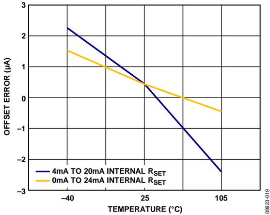
Figure 19. Offset Error vs. Temperature, Internal R<sub>SET</sub> Sense Resistor
