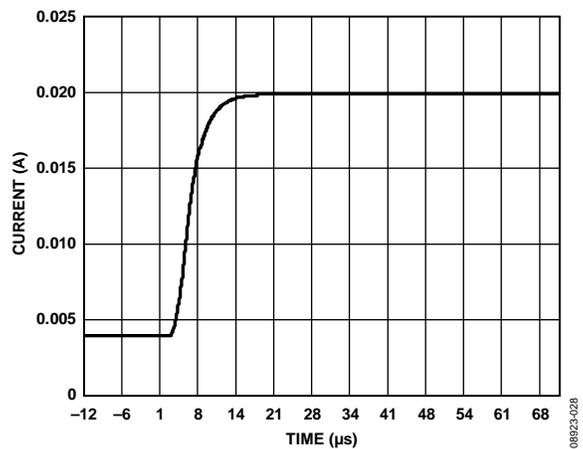
Figure 28. 4 mA to 20 mA Output Current Step
