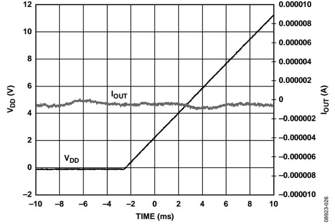
Figure 26. Output Current vs. Time on  $V_{DD}$  Power-Up
