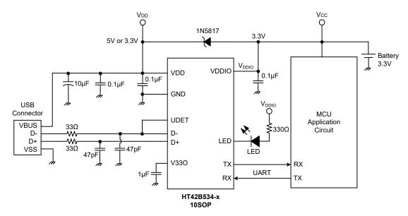
Note: 1. Design note: 10-SOP package only for two power application, the  $V_{\text{CC}}$  power must be below  $V_{\text{DD}}$  power. (The  $V_{\text{CC}}$  power can be from the Li-battery).
