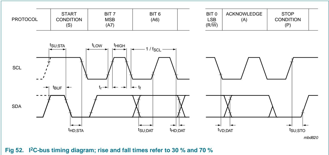
Fig 52. I<sup>2</sup>C-bus timing diagram; rise and fall times refer to 30 % and 70 %
