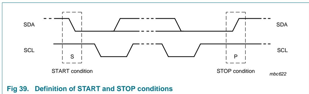
Fig 39. Definition of START and STOP conditions
