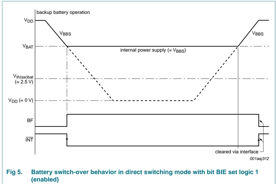
**Fig 5. Battery switch-over behavior in direct switching mode with bit BIE set logic 1 (enabled)**
