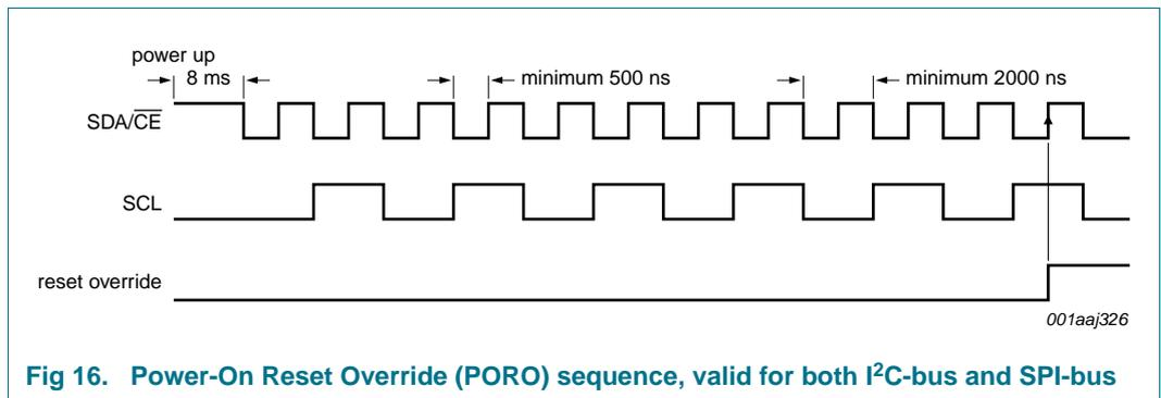
Fig 16. Power-On Reset Override (PORO) sequence, valid for both I<sup>2</sup>C-bus and SPI-bus
