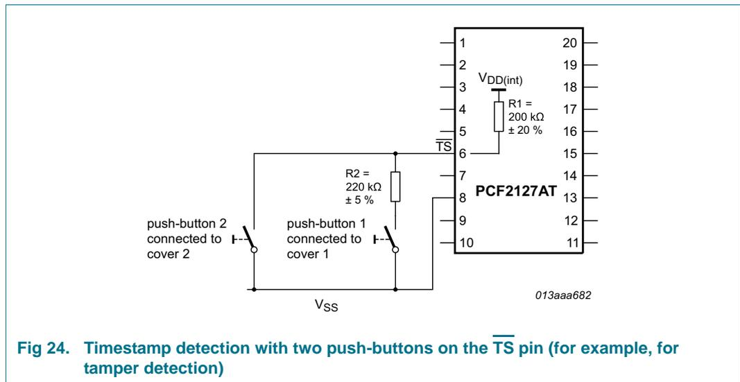
**Fig 24. Timestamp detection with two push-buttons on the  $\overline{TS}$  pin (for example, for tamper detection)**
