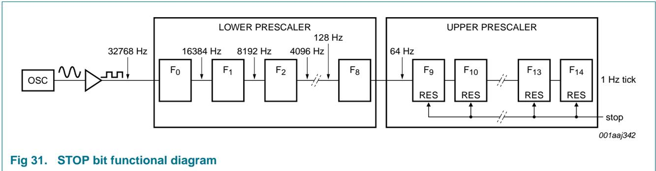
Fig 31. STOP bit functional diagram
