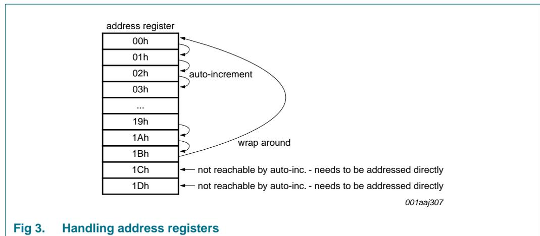
Fig 3. Handling address registers
