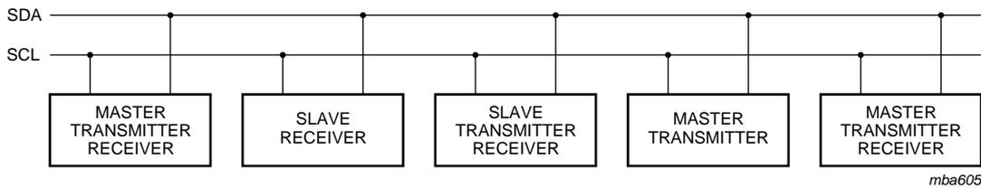
Fig 40. System configuration
