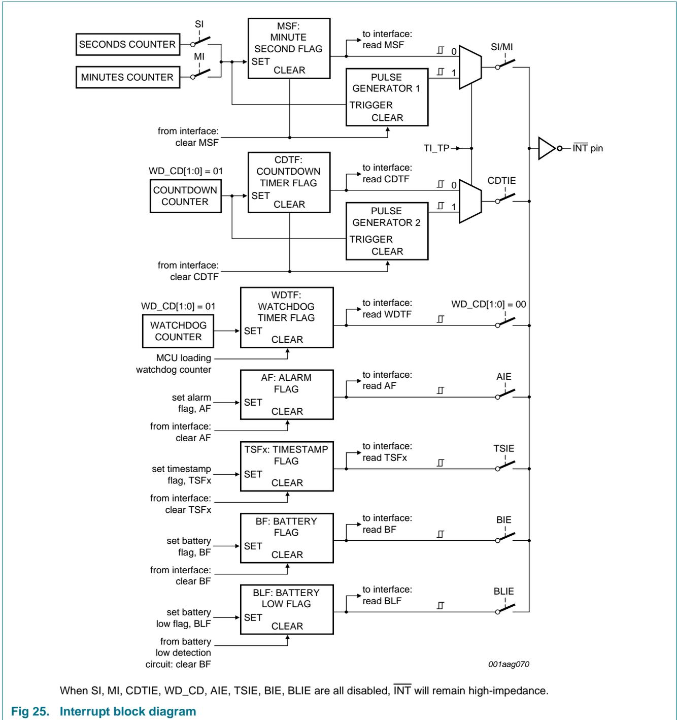
Fig 25. Interrupt block diagram
