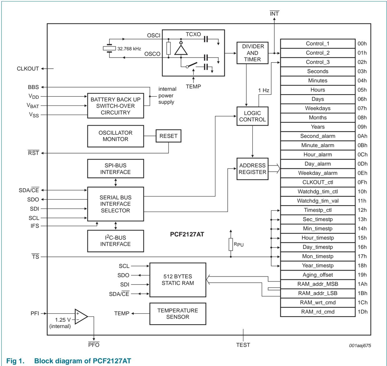
Fig 1. Block diagram of PCF2127AT
