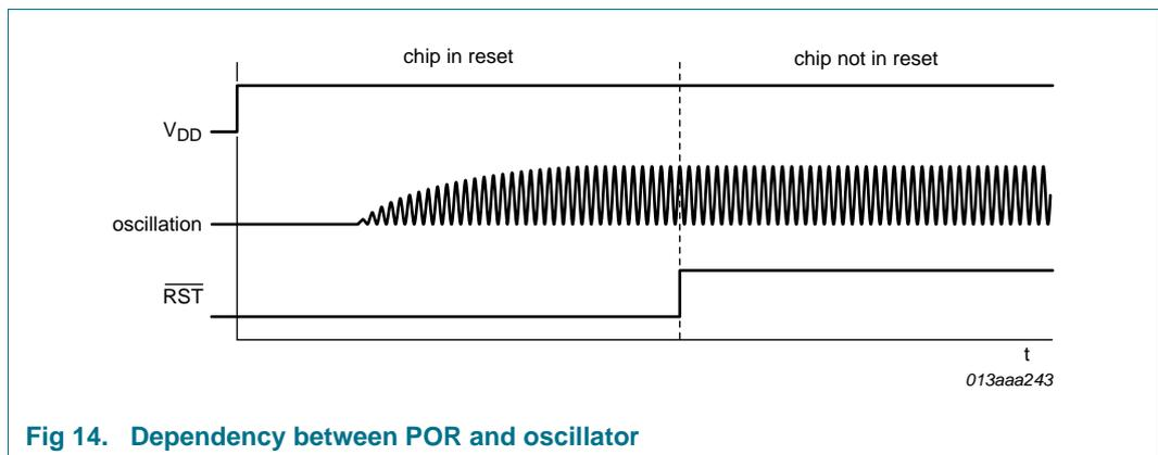
Fig 14. Dependency between POR and oscillator
