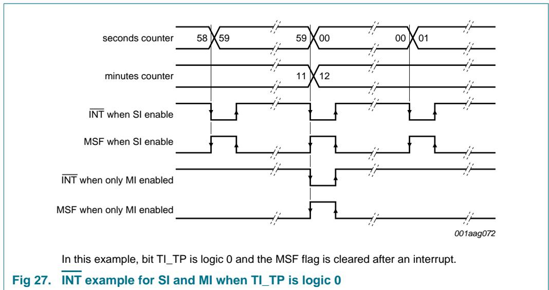
The pulse generator for the minute/second interrupt operates from an internal 64 Hz clock and generates a pulse of  $\frac{1}{64}$  seconds in duration.
