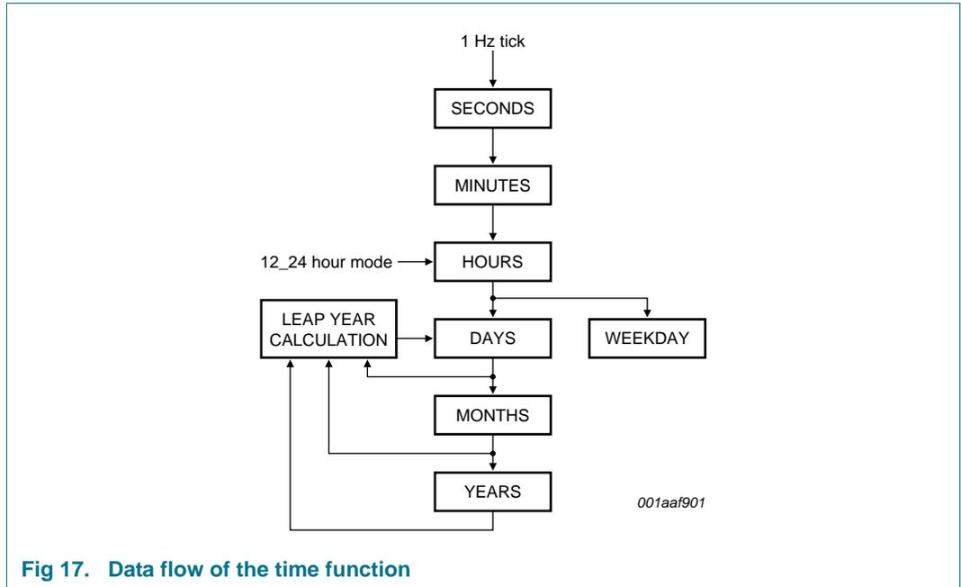
Fig 17. Data flow of the time function
