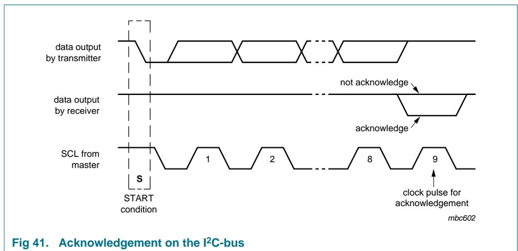
Fig 41. Acknowledgement on the I<sup>2</sup>C-bus
