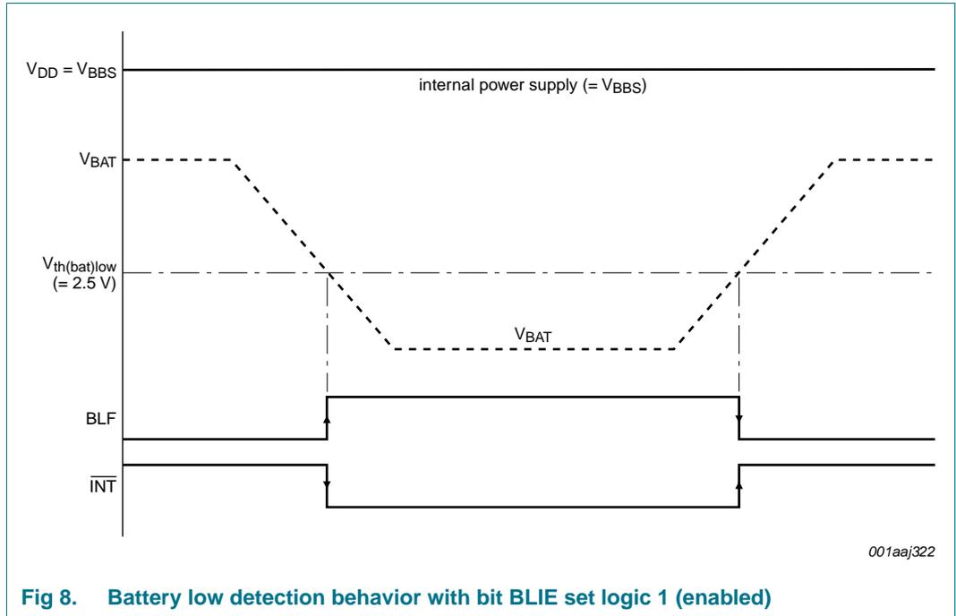
Fig 8. Battery low detection behavior with bit BLIE set logic 1 (enabled)
