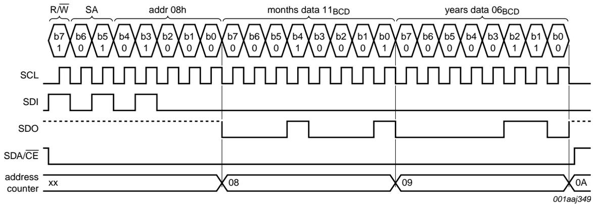
In this example, the registers Months and Years are read. The pins SDI and SDO are not connected together. For this configuration, it is important that pin SDI is never left floating. It must always be driven either HIGH or LOW. If pin SDI is left open, high I<sub>DD</sub> currents may result.
