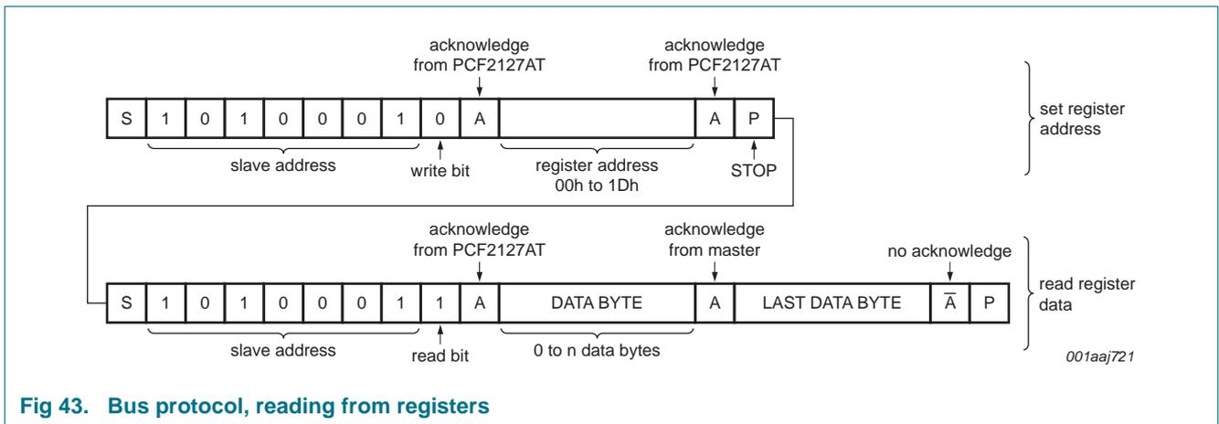
Fig 43. Bus protocol, reading from registers
