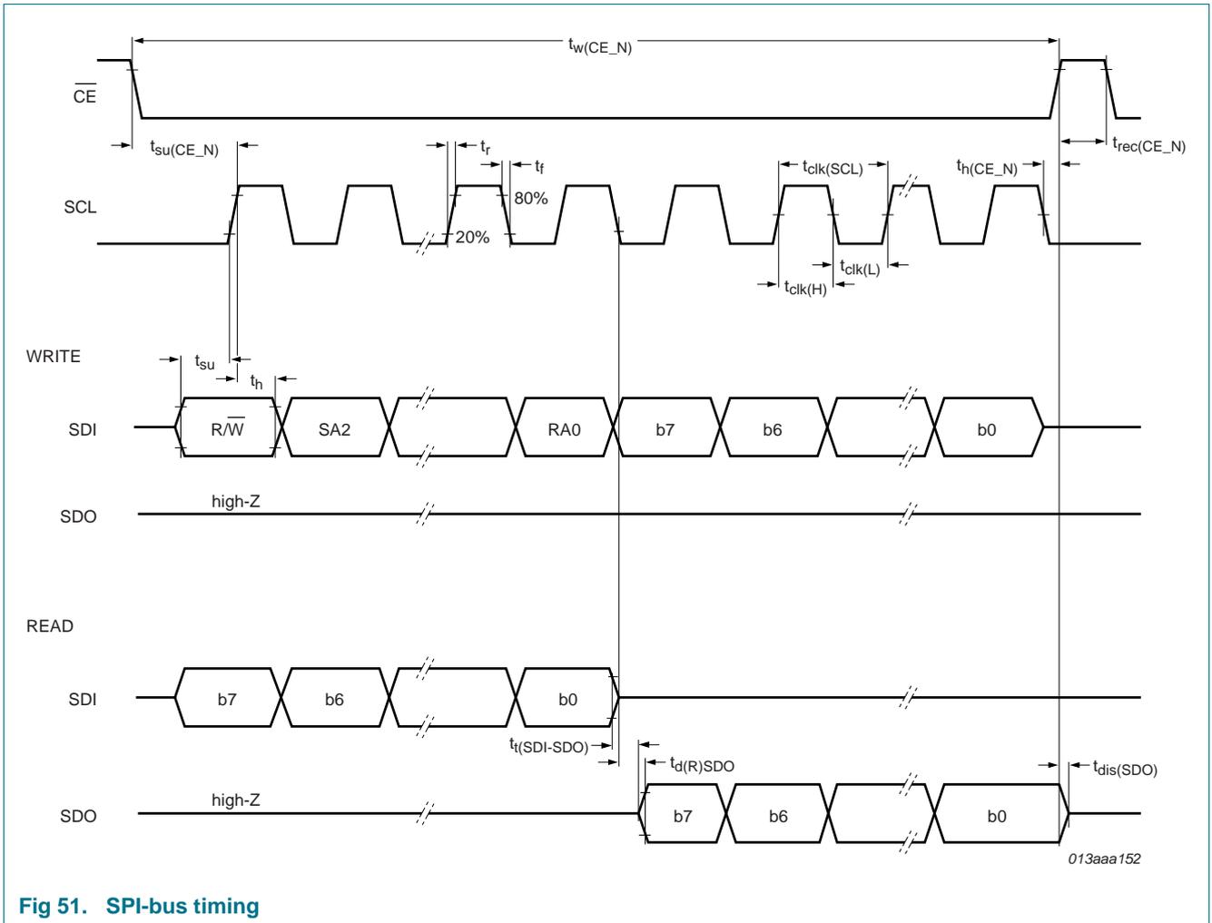
Fig 51. SPI-bus timing
