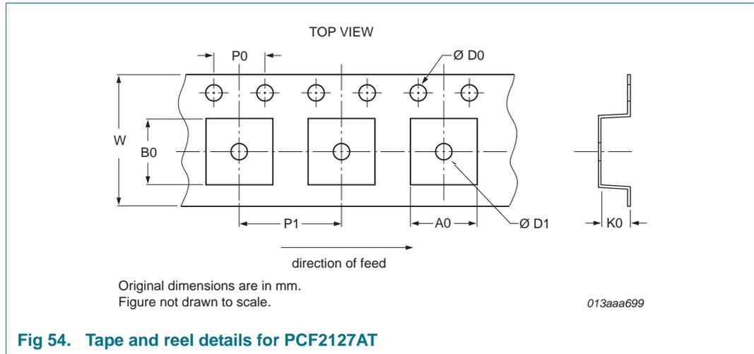
Fig 54. Tape and reel details for PCF2127AT
