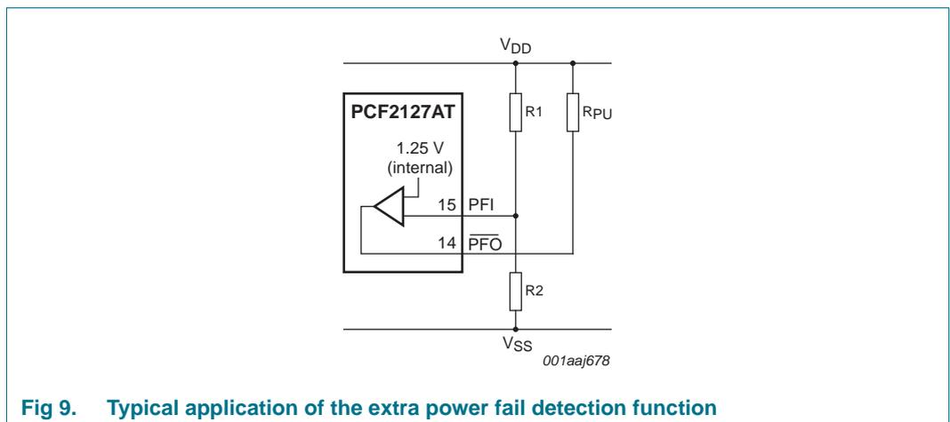
Fig 9. Typical application of the extra power fail detection function
