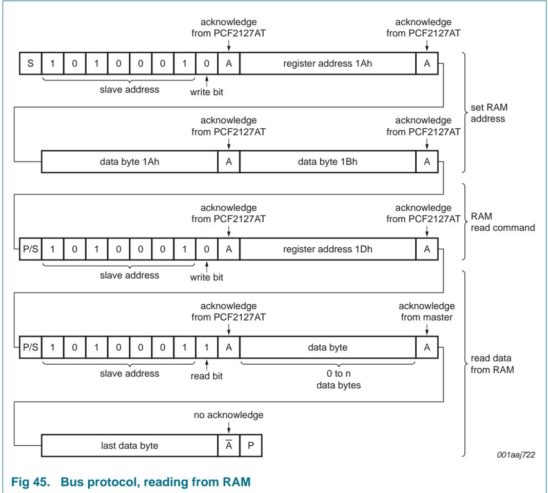
Fig 45. Bus protocol, reading from RAM
