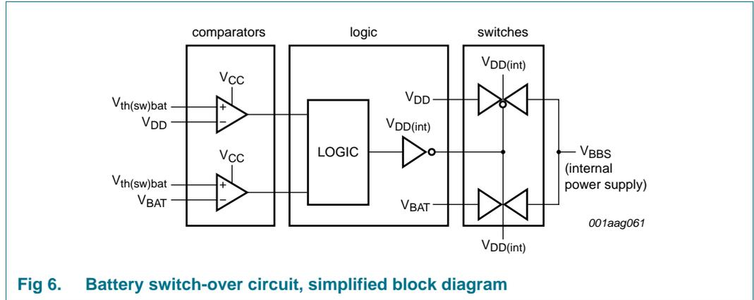
Fig 6. Battery switch-over circuit, simplified block diagram
