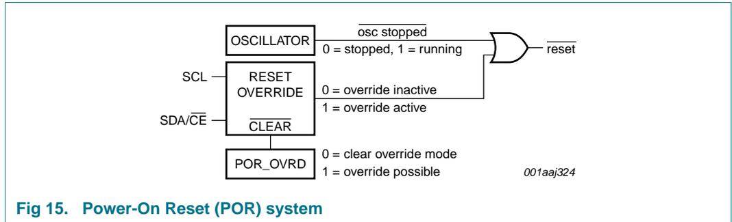
Fig 15. Power-On Reset (POR) system
