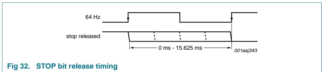
Fig 32. STOP bit release timing
