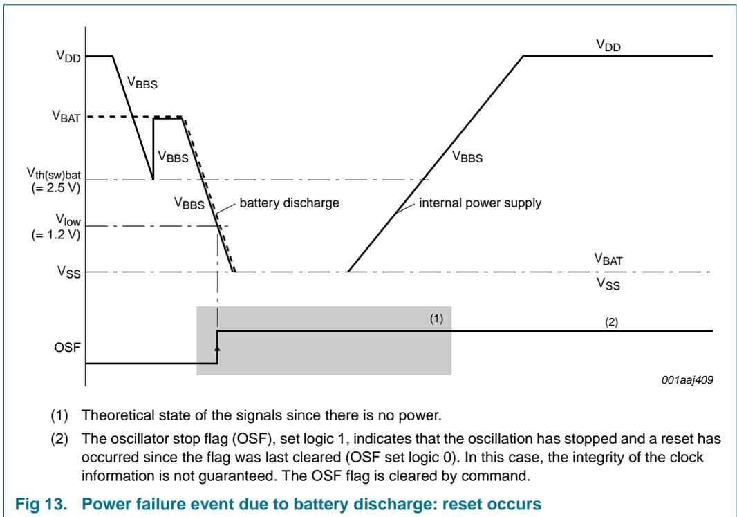
Fig 13. Power failure event due to battery discharge: reset occurs
