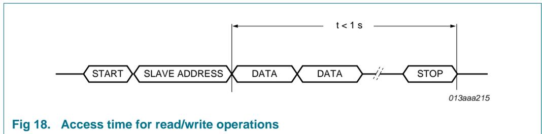
Fig 18. Access time for read/write operations
