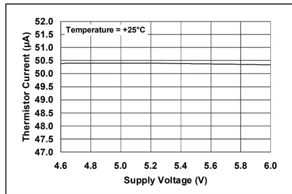
**FIGURE 2-17:** Thermistor Current ( $I_{THERM}$ ) vs. Supply Voltage ( $V_{DD}$ ).
