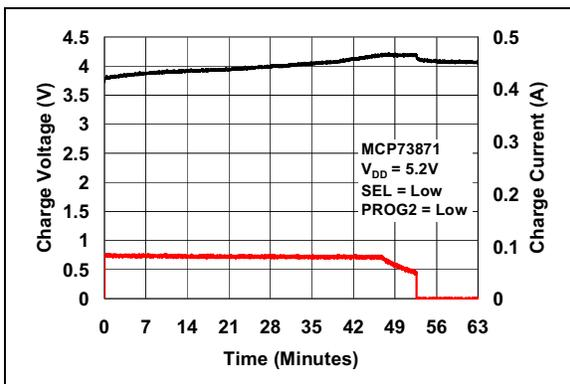
**FIGURE 2-27:** Complete Charge Cycle (130 mAh Li-Ion Battery).
