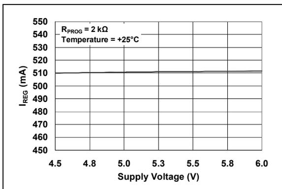
**FIGURE 2-9:** Charge Current ( $I_{OUT}$ ) vs. Supply Voltage ( $V_{DD}$ ).
