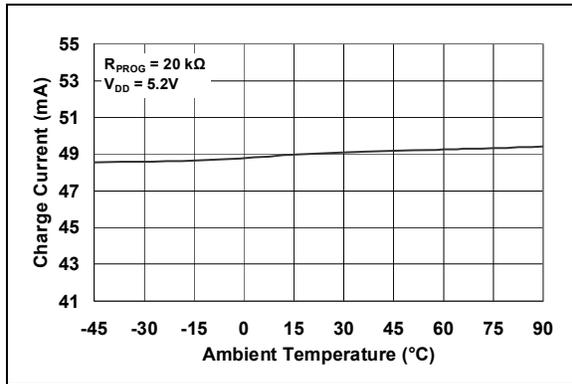
**FIGURE 2-13:** Charge Current ( $I_{OUT}$ ) vs. Ambient Temperature ( $T_A$ ).
