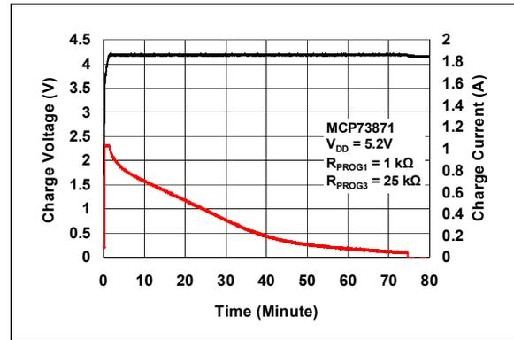
**FIGURE 2-28:** Complete Charge Cycle (1000 mAh Li-Ion Battery).
