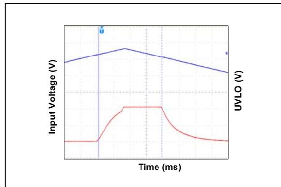
**FIGURE 2-24:** Undervoltage Lockout.
