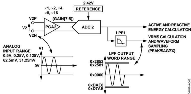
Figure 47. ADC and Signal Processing in Channel 2
