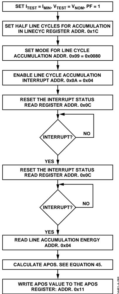
Figure 74. Calibrating Watt Offset with an Accurate Source
