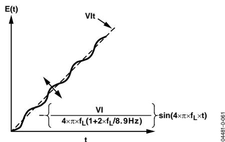
Figure 60. Output Frequency Ripple
