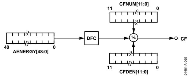
Figure 59. Energy-to-Frequency Conversion
