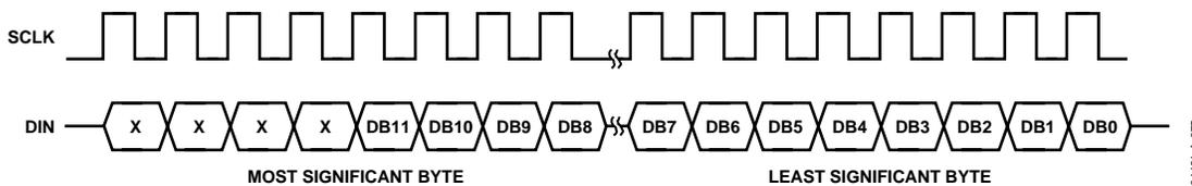
Figure 84. 12-Bit Serial Write Operation
