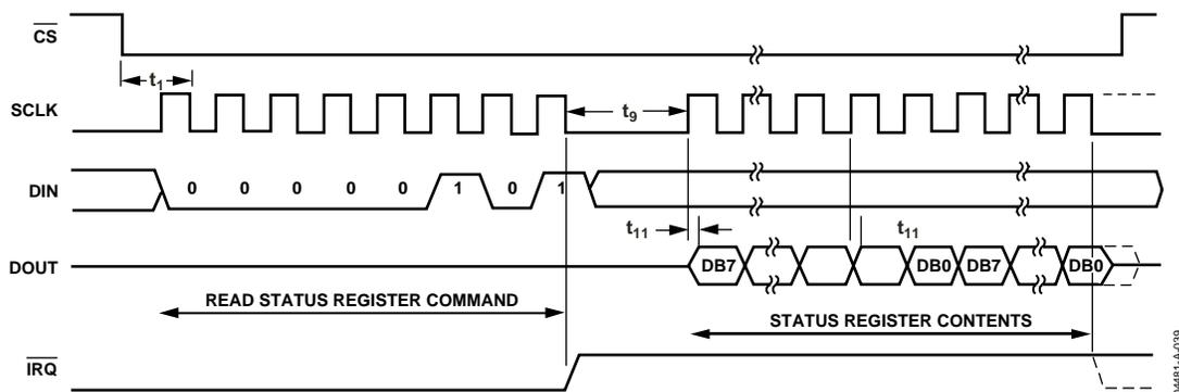
Figure 38. Interrupt Timing
