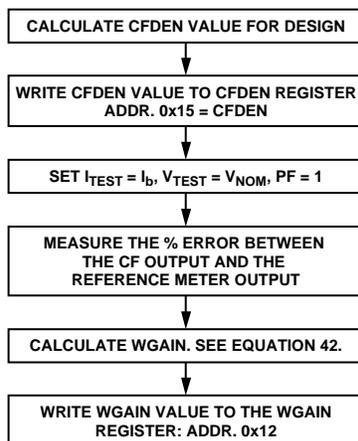
Figure 71. Calibrating Watt Gain Using a Reference Meter
