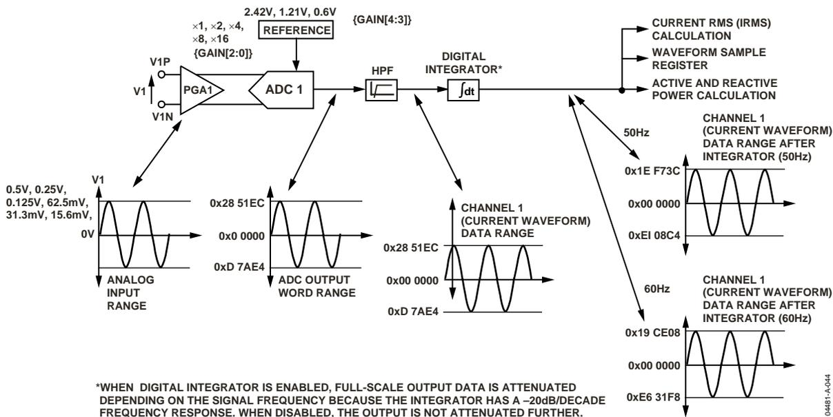
Figure 43. ADC and Signal Processing in Channel 1
