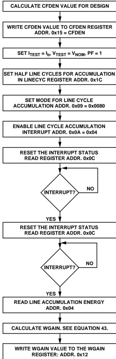
Figure 72. Calibrating Watt Gain Using an Accurate Source
