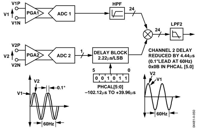
Figure 49. Phase Calibration
