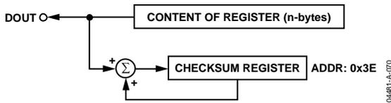
Figure 79. Checksum Register for Serial Interface Read
