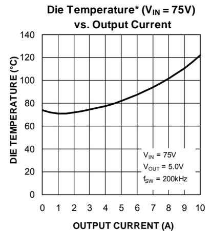
**Die Temperature\*** : The temperature measurement was taken at the hottest point on the MIC2103/04 case mounted on a 5 square inch 4 layer, 0.62", FR-4 PCB with 2oz. finish copper weight per layer, see Thermal Measurement section. Actual results will depend upon the size of the PCB, ambient temperature and proximity to other heat emitting components.
