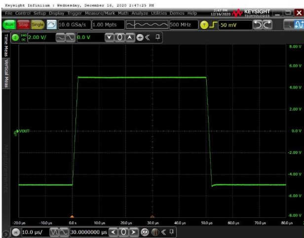
Voltage: 2V/div for Output, Time: 10us/div G=1, VREF = GND; VIN=10VPP, Load R=10K C=100pF Figure 23 Large-Signal Pulse Response
