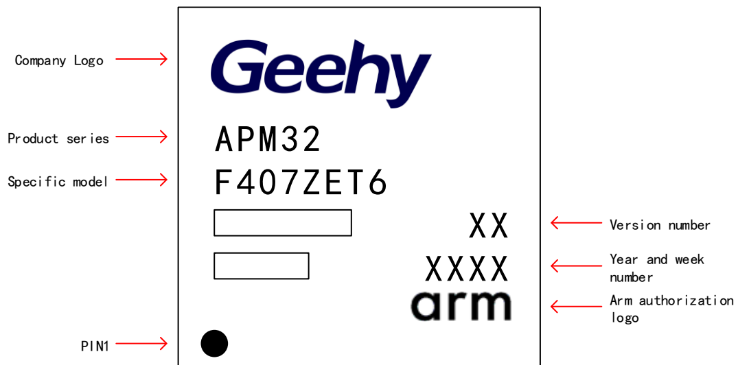
Figure 22 LQFP144 -144 Pins, 20 x20mm Schematic Diagram
