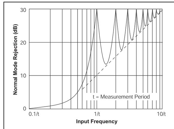
**FIGURE 3-2:** Normal Mode Rejection of Dual Slope Converter
