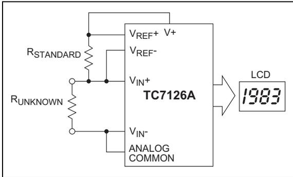
**FIGURE 8-2:** Low Parts Count Ratiometric Resistance Measurement
