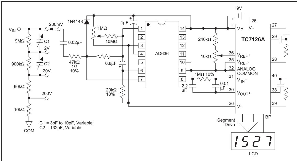
**FIGURE 8-3:** 3-1/2 Digit True RMS AC DMM
