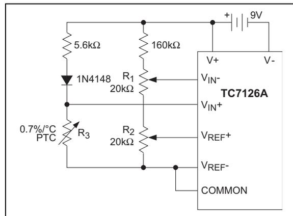
**FIGURE 8-6:** Positive Temperature Coefficient Resistor Temperature Sensor
