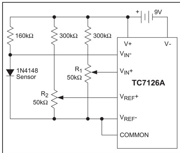
**FIGURE 8-5:** Temperature Sensor
