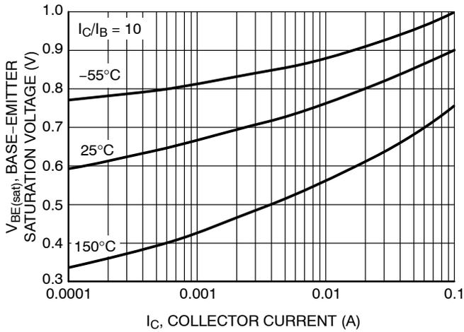
**Figure 3. Base Emitter Saturation Voltage vs. Collector Current**
