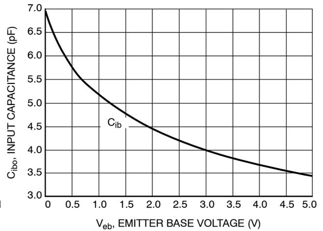
**Figure 6. Input Capacitance**
