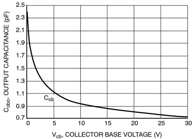
**Figure 7. Output Capacitance**
