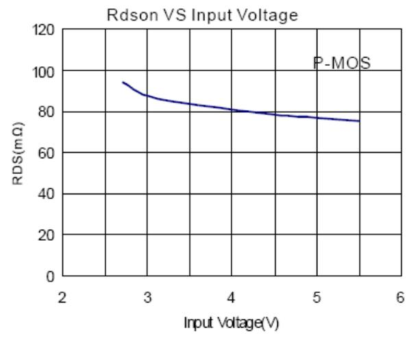
**Typical Performance Characteristics** (Cont.) (@ $T_A = +25^\circ\text{C}$ ,  $C_{IN} = 22 \times 2\mu\text{F}$ ,  $C_O = 22\mu\text{F}$ , unless otherwise specified.)
