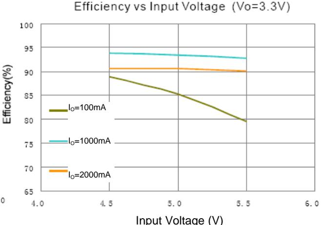
**Typical Performance Characteristics** (Cont.) (@ $T_A = +25^\circ\text{C}$ ,  $C_{IN} = 22 \times 2\mu\text{F}$ ,  $C_O = 22\mu\text{F}$ , unless otherwise specified.)
