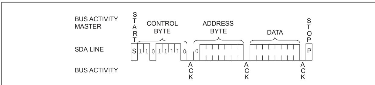
**FIGURE 6-2: SRAM/RTCC SEQUENTIAL WRITE**
