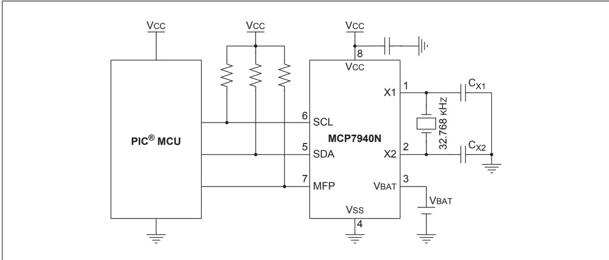
**FIGURE 1-2: BLOCK DIAGRAM**
