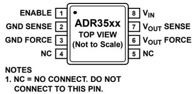
Figure 2. Pin Configuration
