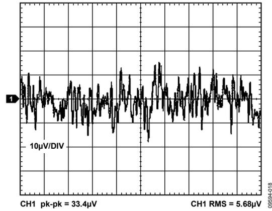
Figure 18. ADR3550 Output Voltage Noise (0.1 Hz to 10 Hz)
