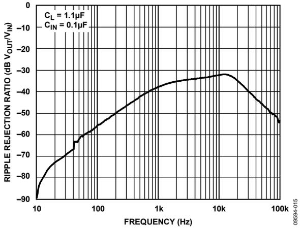
Figure 15. ADR3525 Ripple Rejection Ratio vs. Frequency
