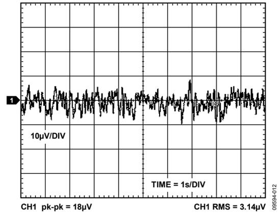
Figure 12. ADR3525 Output Voltage Noise (0.1 Hz to 10 Hz)
