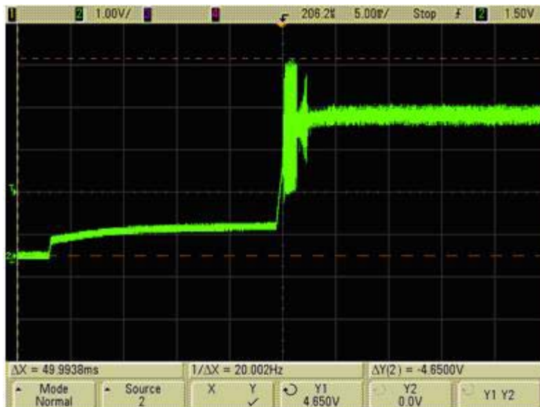
Figure 13. Input Voltage Overshoot >4V (Bad)
