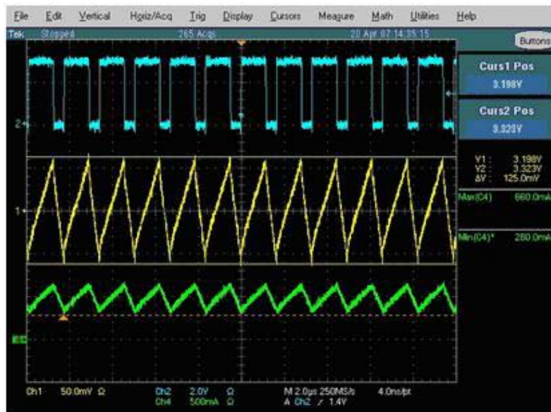
Figure 21. Electrolytic 100 \mu F (Ripple Too High)
