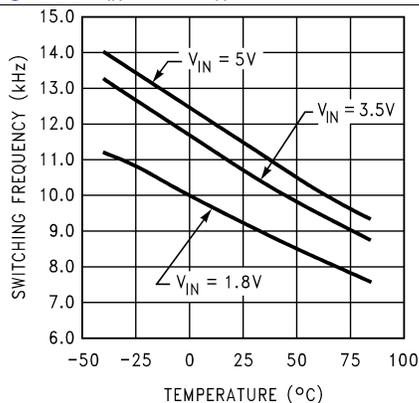
Figure 7. Switching Frequency vs Temperature
