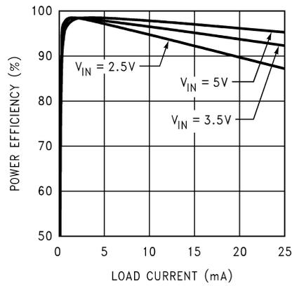
Figure 15. Efficiency vs Load Current
