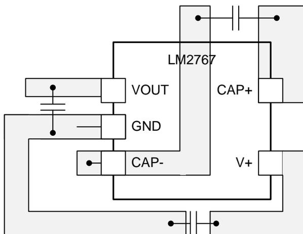
**Figure 16. LM2767 Layout Example**
