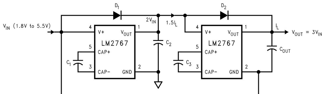
Figure 13. Increasing Output Voltage By Cascading Devices
