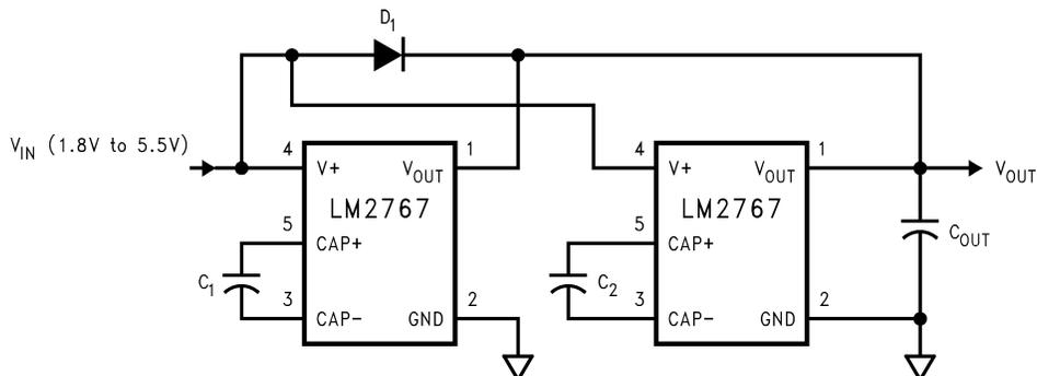
Figure 12. Lowering Output Resistance by Paralleling Devices
