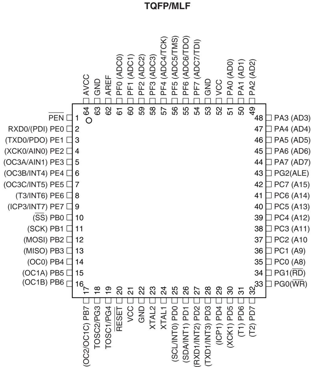
Note: The bottom pad under the MLF package should be soldered to ground.
