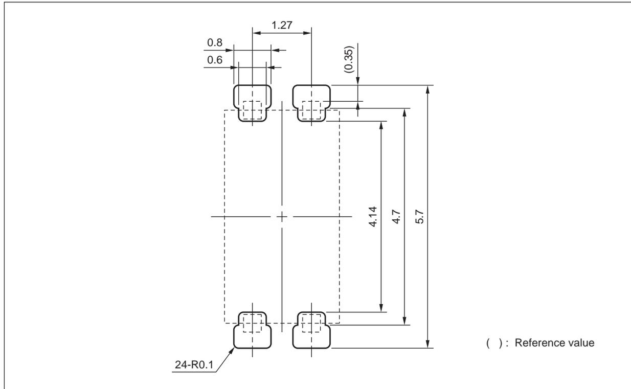
**Remark** This drawing is considered to meet air and outer creepage distance 4.0 mm minimum. All dimensions in this figure must be evaluated before use.
