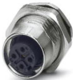
Sensor/actuator flush-type socket, 5-pos. with shield contact, M12 SPEEDCON, A-coded, rear/screw mounting with M16 thread, with straight solder connection
